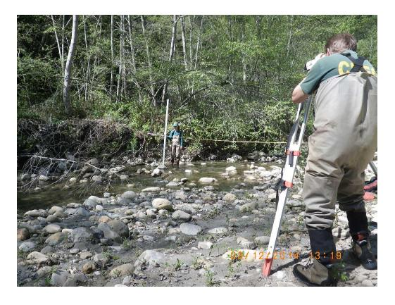
Primarily used to estimate hydraulic characteristics over a range of flows (average depth, average velocity, wetted perimeter, and hydraulic radius).
