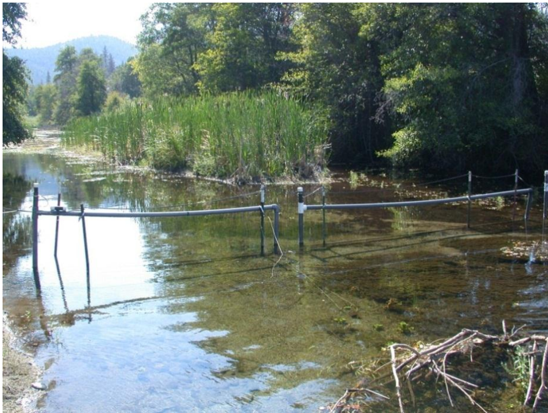
Figure 5: A single PIT array consisting of four antennas spanned the channel approximately 93 m above the mouth of Sugar Creek. The unique PIT tag codes identified individual fish passively as they move near the antenna array. Photograph by M. Olswang, Sept. 2011.
