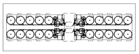
Figure 5.4: Rearing tanks and recirculation systems at the Satellite Incubation and Rearing Facility
