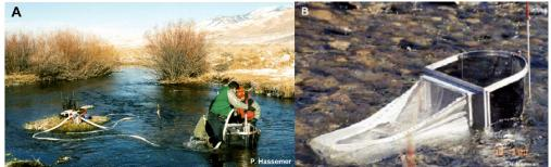
Figure 7.1: Sample of Hydraulic Redd Pumping (From Venditti et al. 2002b)
