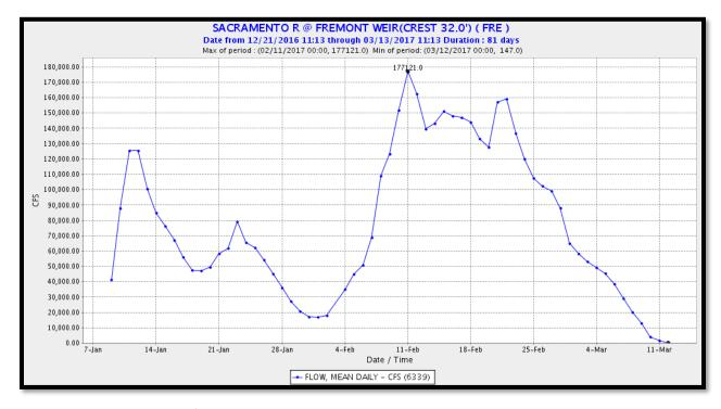
**Figure 8.** Hydrograph of Fremont Weir 62-day Overtopping Event, 9 January through 12 March 2017. Mean daily flow during the period was 78,649 cubic feet per second.
