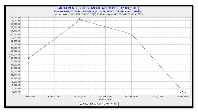
**Figure 7.** Hydrograph of Fremont Weir 4-day overtopping event, 17 through 20 December 2016. Mean daily flow during the period was 18,105 cubic feet per second.
