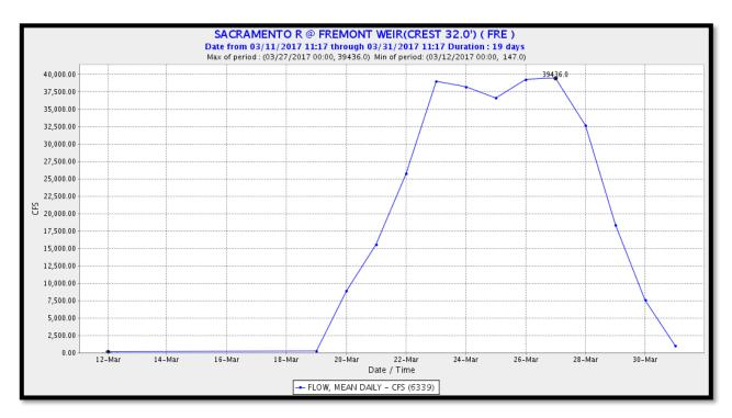
**Figure 9.** Hydrograph of Fremont Weir 13-day Overtopping Event, 19 through 31 March 2017. Mean daily flow during the period was 23,281 cubic feet per second.
