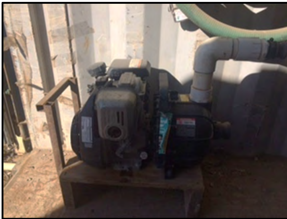
Figure 23. Pump used to Operate the Clam Rake
