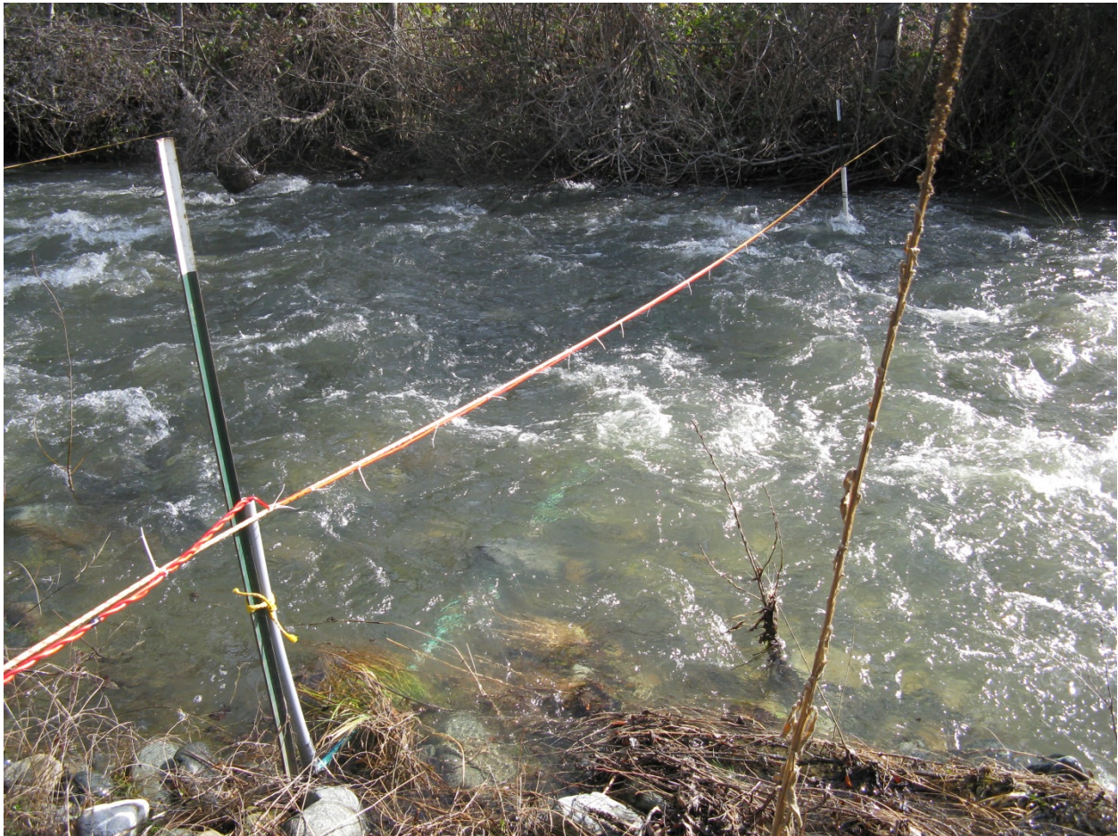
Figure 2. Photo of the upstream antenna at the Rush Creek tributary PIT monitoring site.
