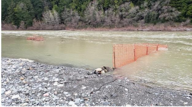
14.) 01.29.2020. Camera setup near maximum operational capacity. Rock wall constructed is approximately where 9,000 cfs brings water level to.
