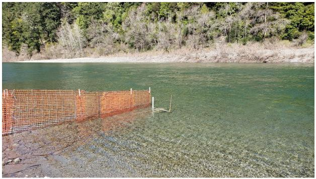
19.) 03.02.2020. Camera setup pictured showing clarity of low flow in March during steelhead run. Streamflow 392 cfs at Ft. Seward USGS gage.
