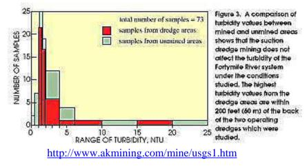
In American studies, average turbidity levels have been shown to be between 5 and 15 NTU 5 meters below dredges. But even the maximum turbidity level measured in a clay pocket (51 NTU) fell below 10 NTU within 45 meters. Turbidity increases, from even large dredges on moderate sized streams, have shown to be fairly low, usually 25 NTU or less, and to return to background within 30 meters. The impact is localized and short lived; indicating minimum impact on moderate and larger waterways.
