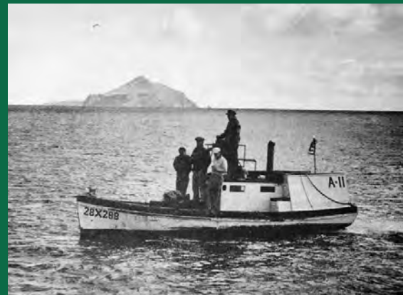
1950—The Mollusk , a 26-foot research vessel, supported marine surveys off California's southern and central coasts. Based in San Pedro, the small, wooden vessel was often towed to dive sites by larger mother ships to support the diving operations.
