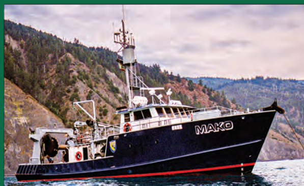
1990—The Mako , an 80-foot, long-range steel hulled trawler, custom built with A-frame, dual winches and doors for mid-water bottom trawling and longline research fishing. Transferred in 2009 to the California Maritime Academy as a training vessel.
