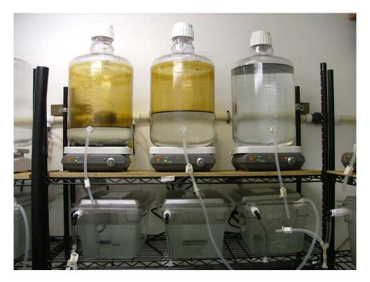
Figure 24 . 20-L polycarbonate carboys used for WAF and CEWAF preparation (above) and 18-L polycarbonate aquaria used for smolt exposures (below).
