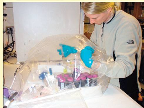
USGS's Jennifer Agee sampling sediment in an anoxic glove bag.
