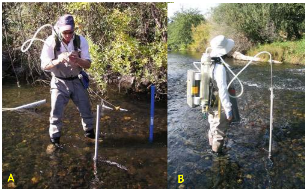
Figure 9. Measuring permeability in spawning riffles of the Sacramento River. (A) Permeability standpipe and sipping rod. (B) Permeability backpack.
