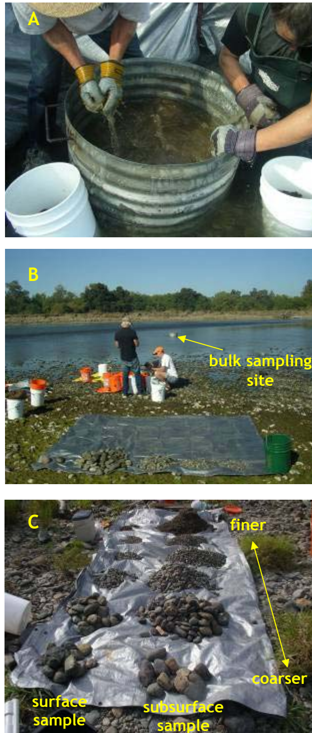
Figure 8. Bulk sampling of surface and subsurface bed samples from the Sacramento River. (A) A section of culvert (30 inch diameter) is worked into the bed and particles from the surface are extracted by hand. (B) Samples are sieved and the mass of each size class is recorded on a nearby bank. (C) Surface (left) and subsurface (right) samples, segregated into size classes for one of the samples from the middle Sacramento River.
