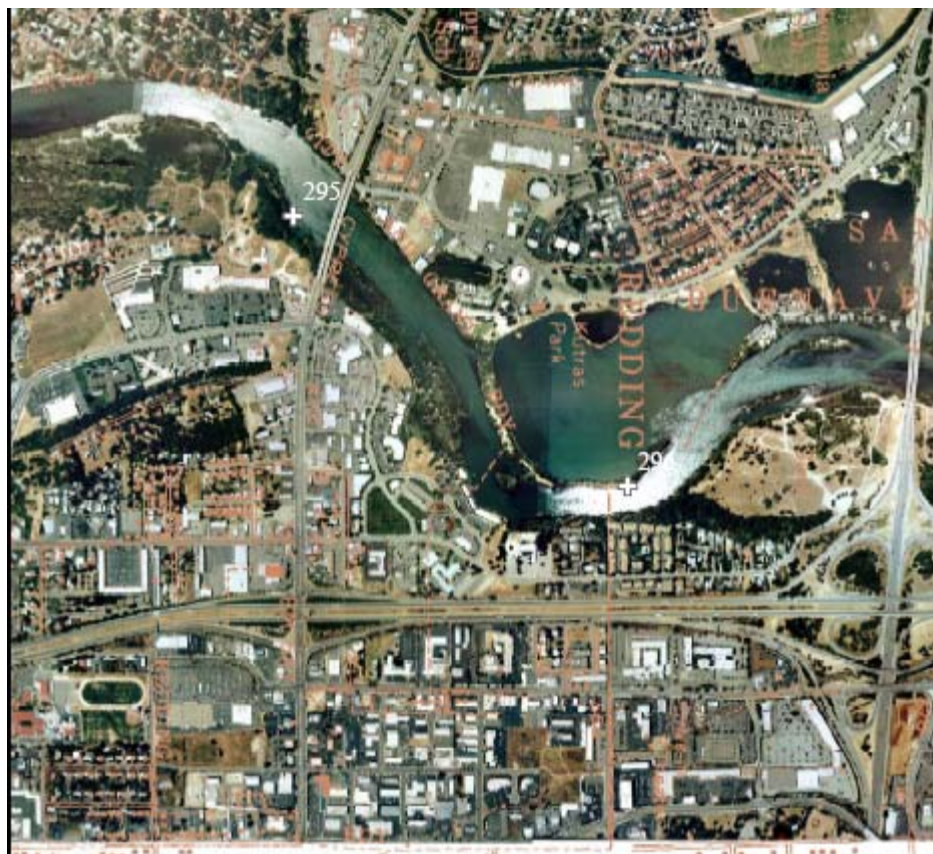
Figure 1. Lasting effects of aggregate extraction. Kutrass Park (center) was one of the primary borrow areas for aggregate to support Shasta and Keswick dam construction. More than 7 million cubic yards of sediment was mined from the upper Sacramento River basin, much of it from the mainstem channel and floodplain. Remnant mining pits can function as sediment traps
