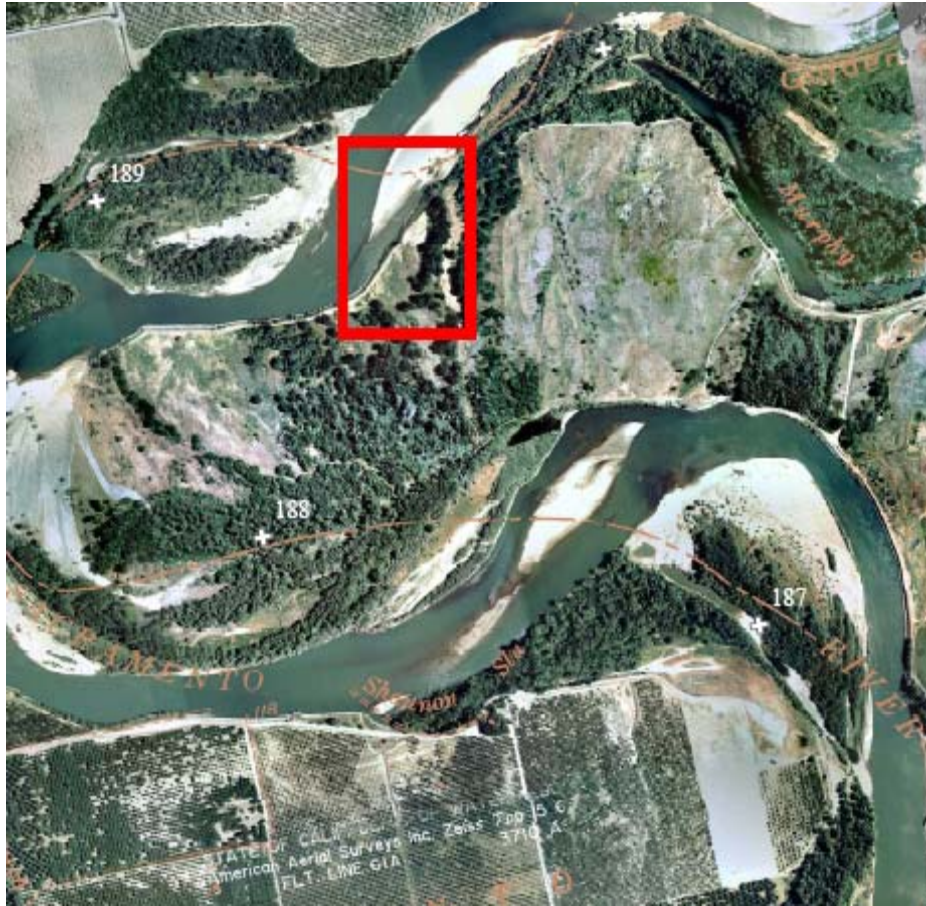
Figure 2. Example of a scour channel that forms on the downstream end of a point bar. (Photo Source: CDWR 1999)
