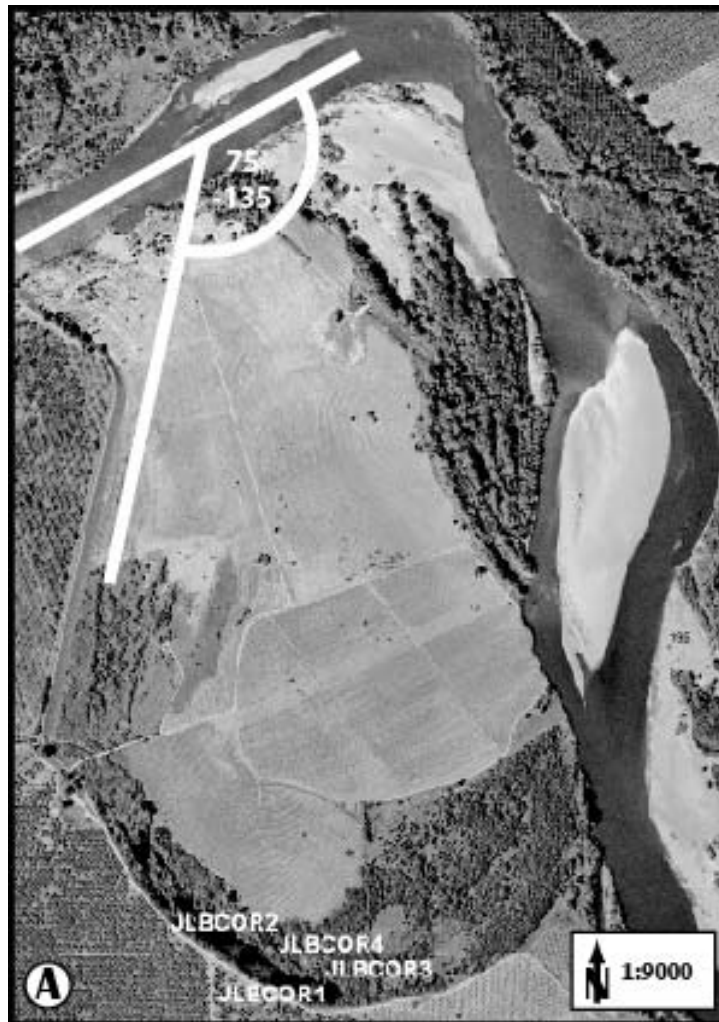
Figure 55. (A) Aerial photo of Jenny Lind Bend near river mile 195 taken in 2004. The diversion angle and core locations are shown within the photo. (B) Granulometric profile for core JLBCOR4.
