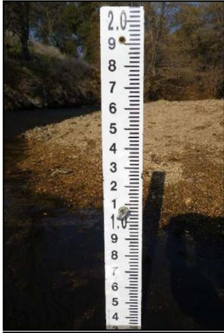
Figure 7. Example of staff gage used to monitor change in flow conditions.
