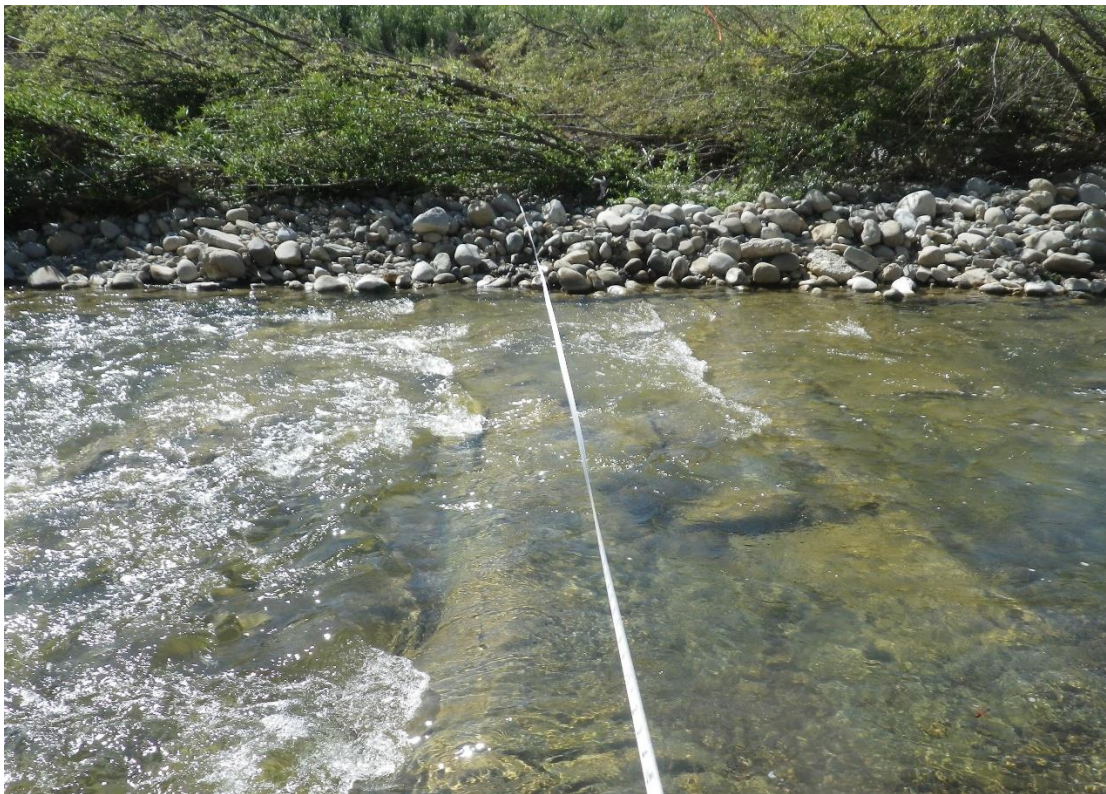
Figure 5. Example of a transect across the hydraulic control at the top of a riffle. Stream is flowing from right to left.
