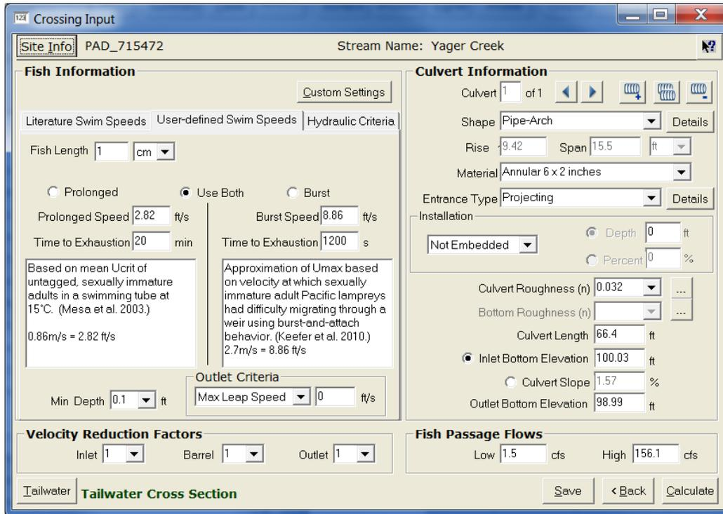
Figure 3-3. Example of FishXing user interface where model parameters are entered.
