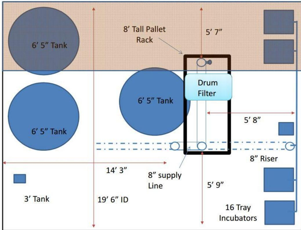
Figure 2. Current layout of facilities in the fisheries shed at the Interim Facility.
