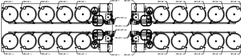
Figure 6. Recirculation and chiller for translocation and rearing – Concept Design
