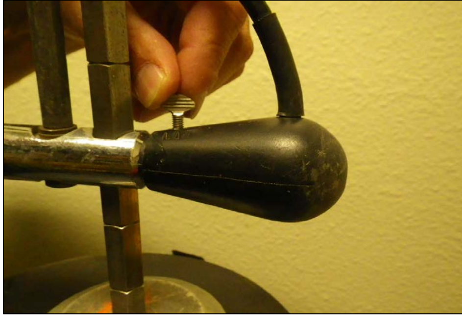
Figure 4: Attaching Probe of Model 2000 attached to the wading rod using wing screw.
