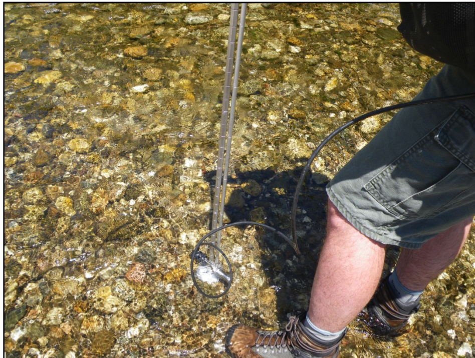
Figure 5: Probe of Model 2000 attached to the wading rod.
