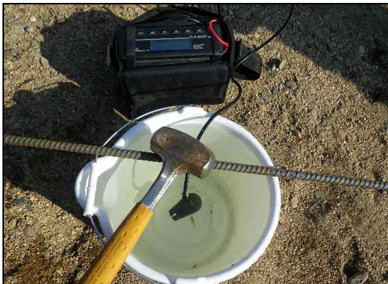
Figure 2: Set up for calibration of the Model 2000 flow meter. This example shows the probe suspended from the rebar, and stabilized by the hammer.
