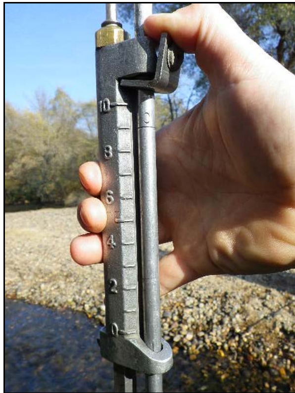
Figure 6: USGS Top-Setting Wading Rod handle showing vernier scale set at 0.9 ft.
