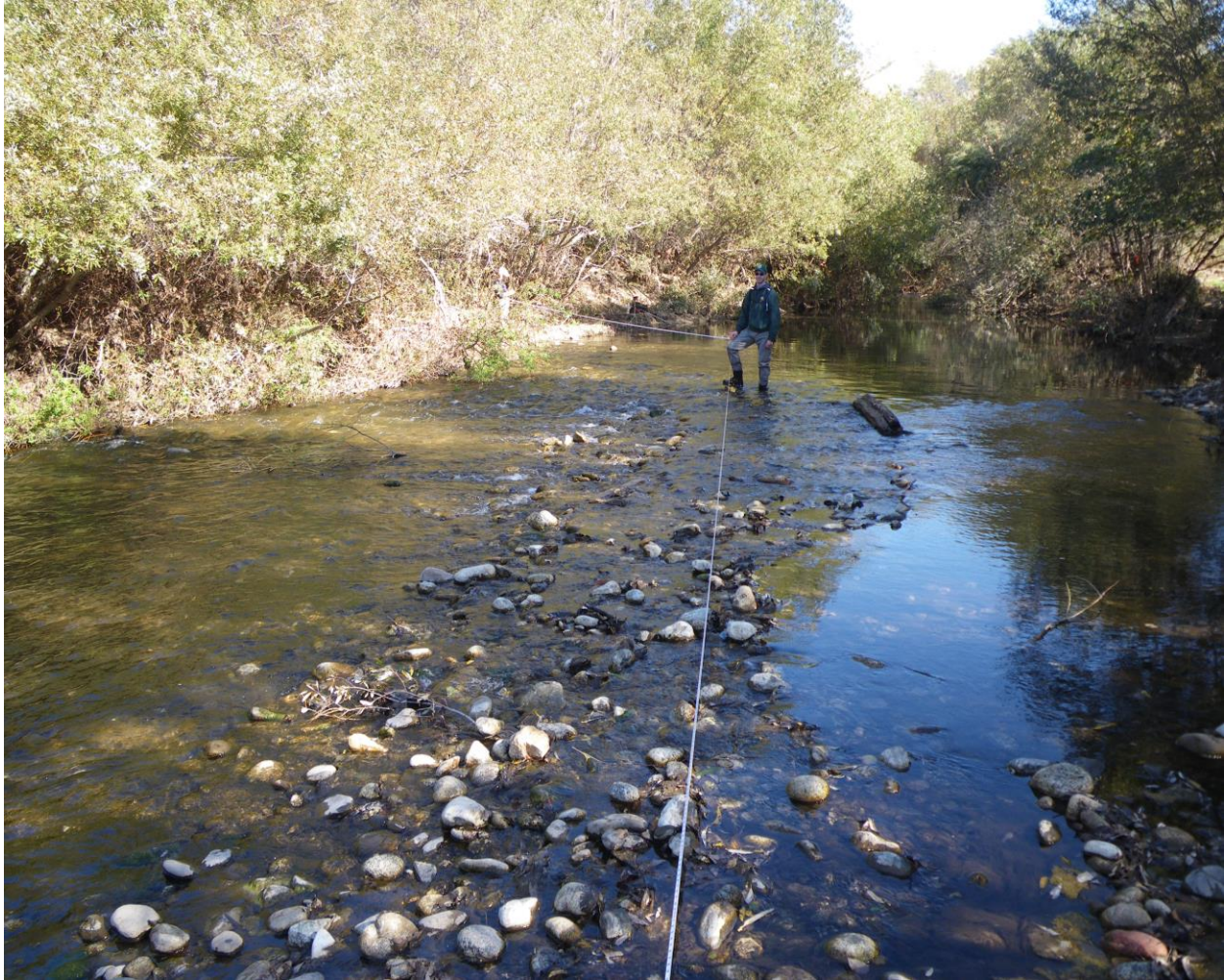
Figure 1. Example of a critical riffle transect that follows the shallowest course from bank to bank
