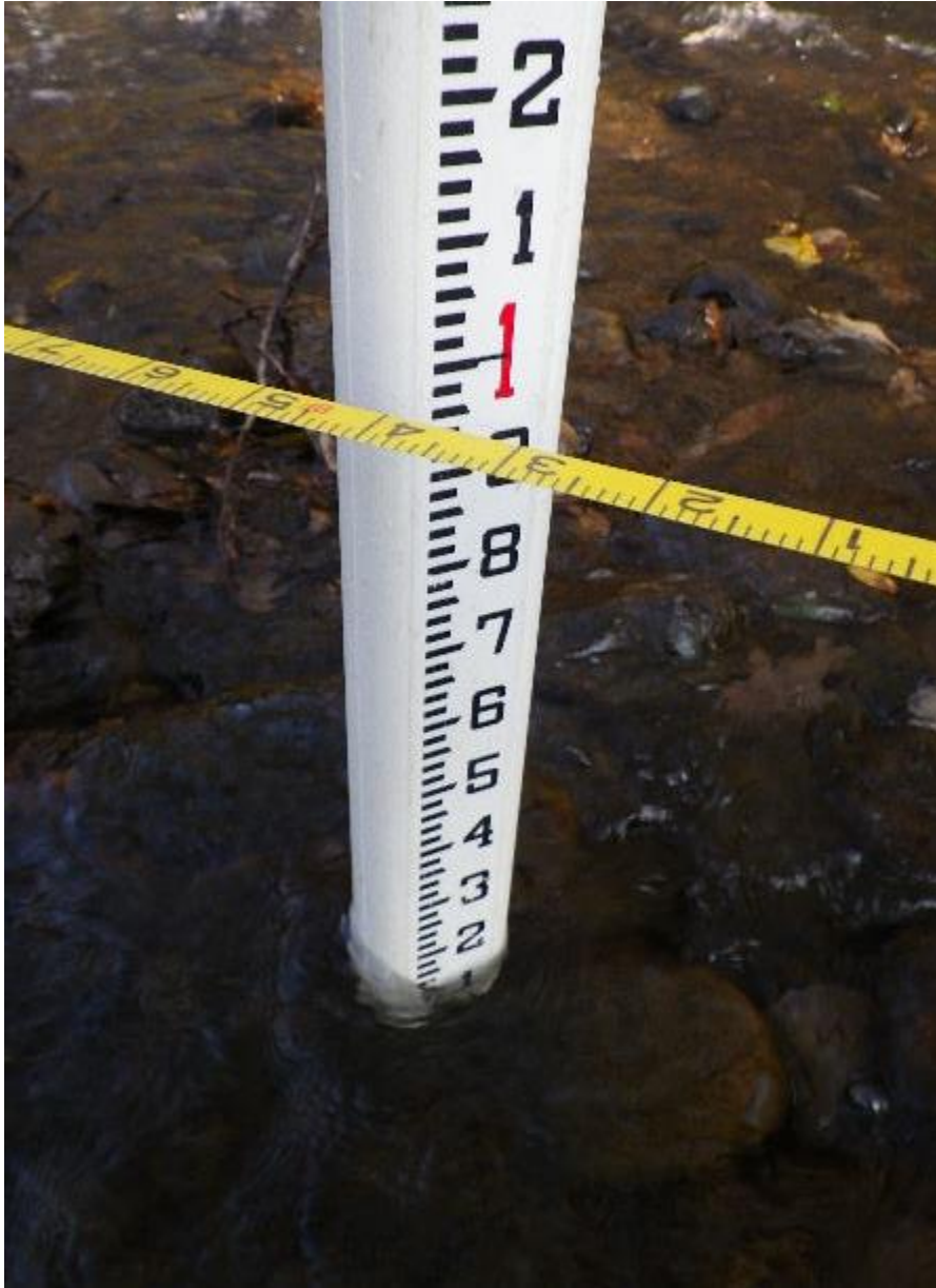
Figure 3. Detail: Using the stadia rod to measure depth along a critical riffle transect
