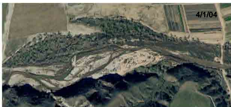
Figure 6. Progression of aerial photographs downstream of Castaic Canyon, showing channel change between 1993 and 2005. Note that there was little change between 2000 and 2004, but the active corridor widened significantly in response to the 2005 events, and that channel traces within the active corridor were effectively erased. See appendix A for photo sources.
