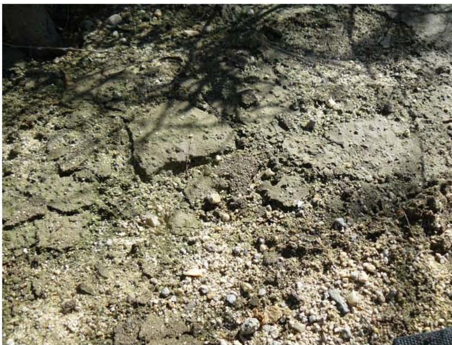
Photo 8. A view of wetland hydrology indicators including soil cracking, crust, and sediment deposits. This photo was taken on September 25, 2007 (PC-15).
