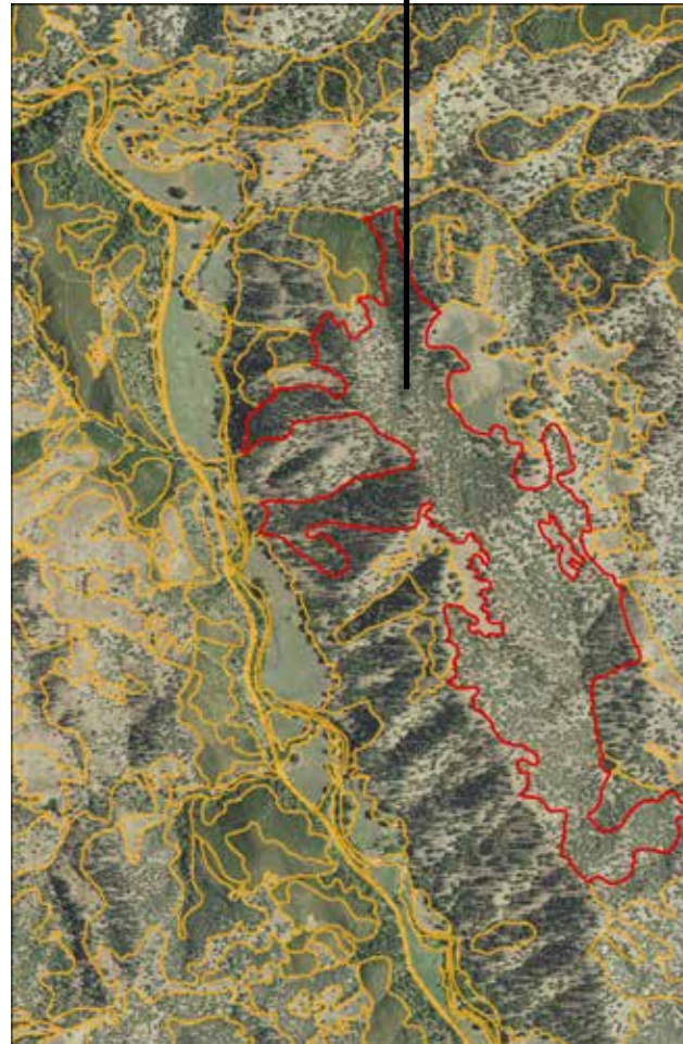
FIGURE 2 Example of an SCV GIS layer derived from detailed aerial imagery and field samples. This map shows vegetation polygons drawn over aerial imagery. The finely detailed polygons are delineated based on type of vegetation and value of vegetation cover. The table on the left shows some of the robust attributes associated with the SCV polygon outlined in red.
