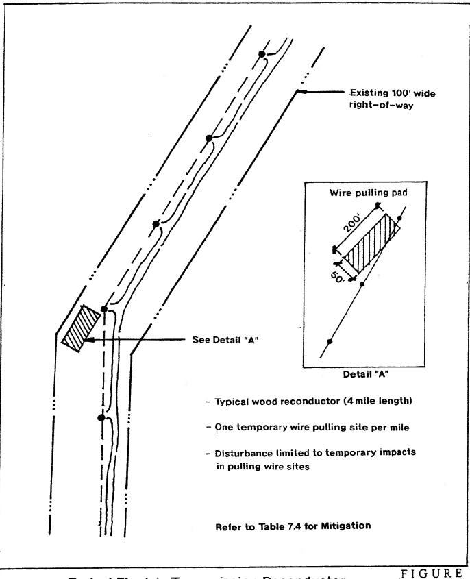
Typical Electric Transmission Reconductor in Existing R/W (Wood)
