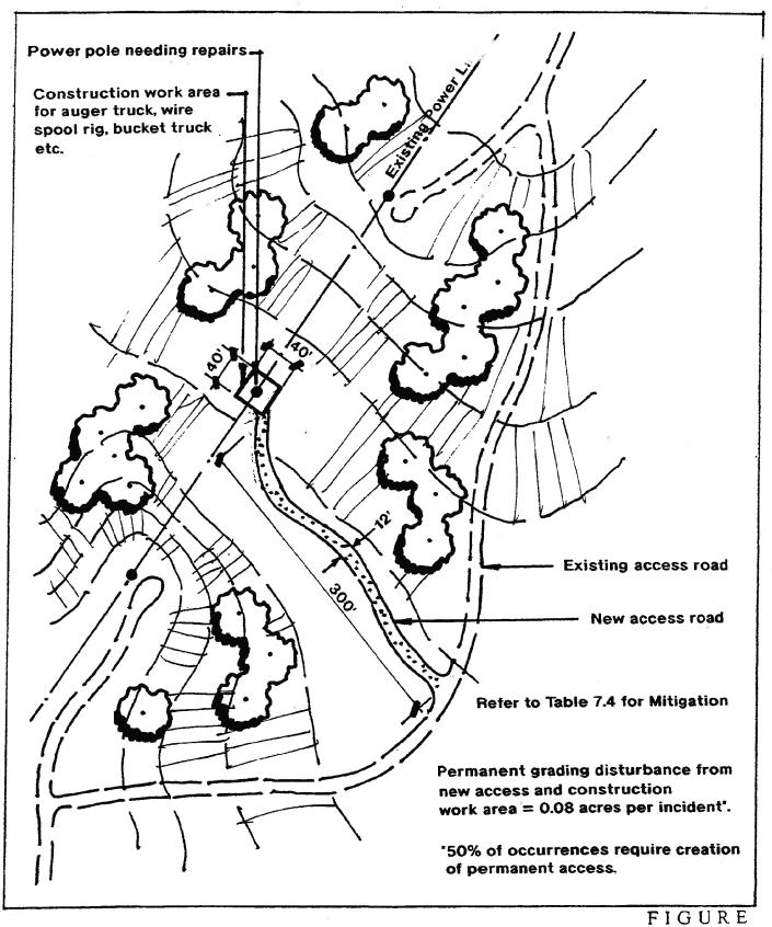
Typical Electrical Transmission or Distribution Repairs
