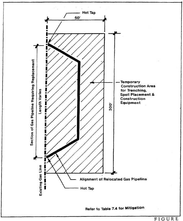
Typical Gas Pipeline Relocation Impact Diagram
