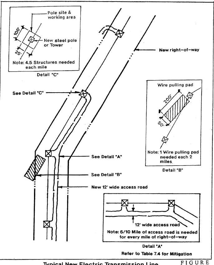
Typical New Electric Transmission Line Requiring New R/W (Steel)
