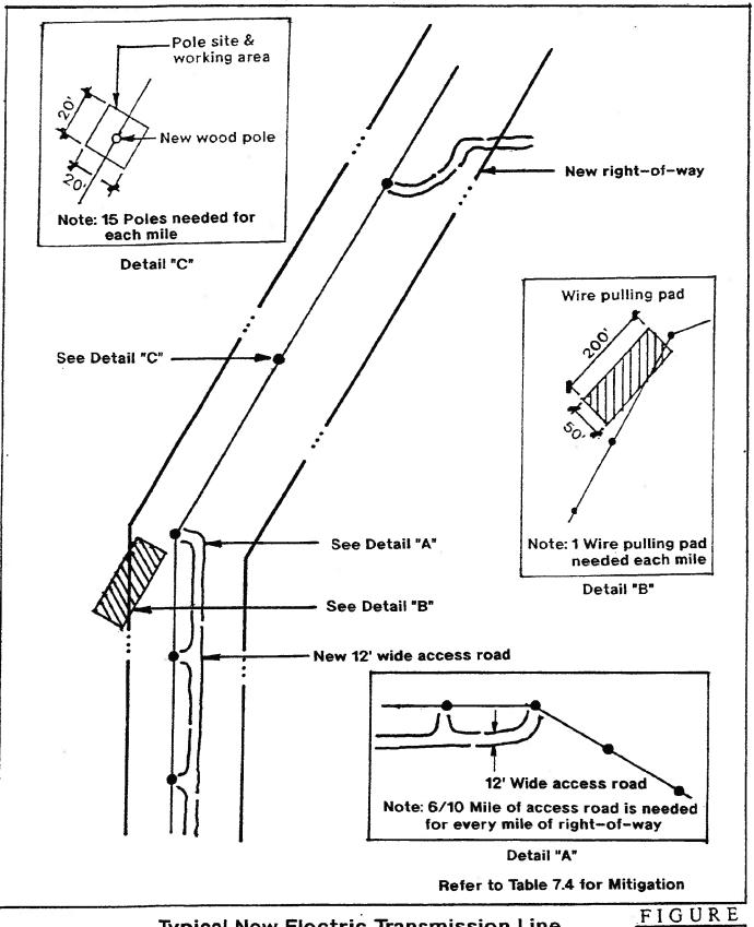
Typical New Electric Transmission Line Requiring New R/W (Wood)
