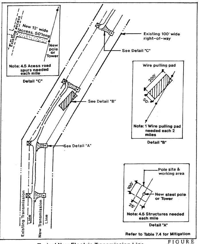
Typical New Electric Transmission Line in Existing R/W (Steel)
