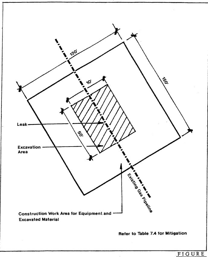
Typical Corrective Action to Repair Gas Pipeline Leak
