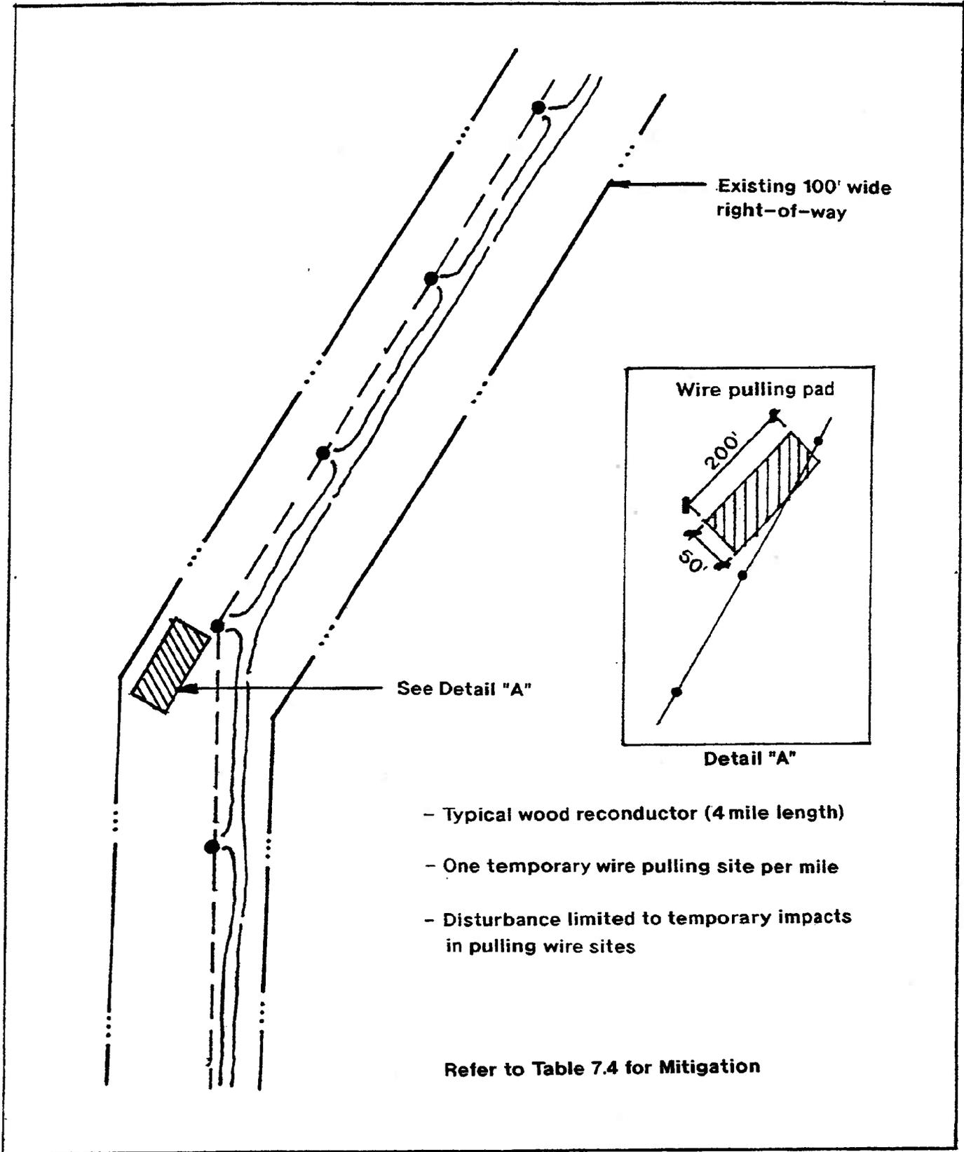
**Typical Electric Transmission Reconductor
