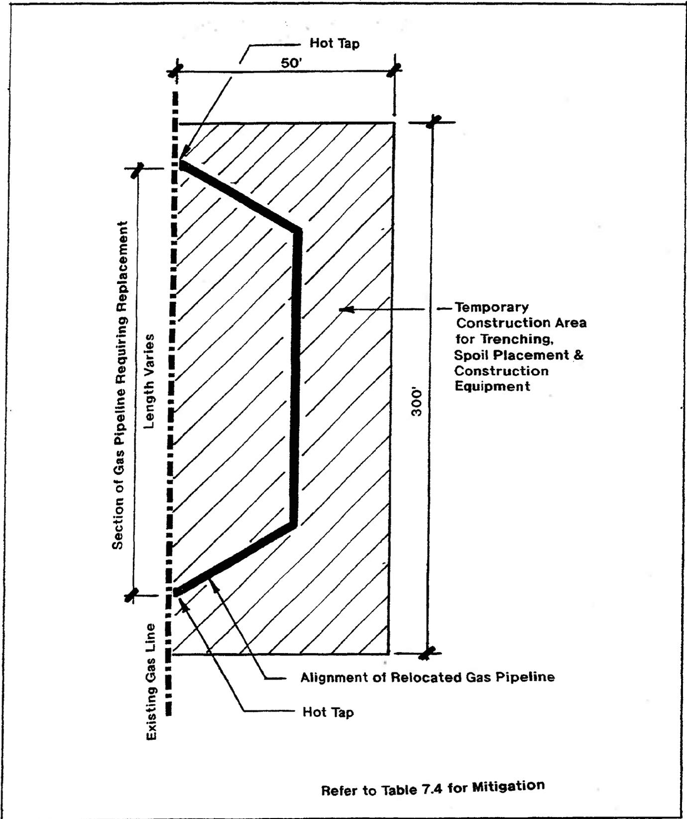
Typical Gas Pipeline Relocation Impact Diagram
