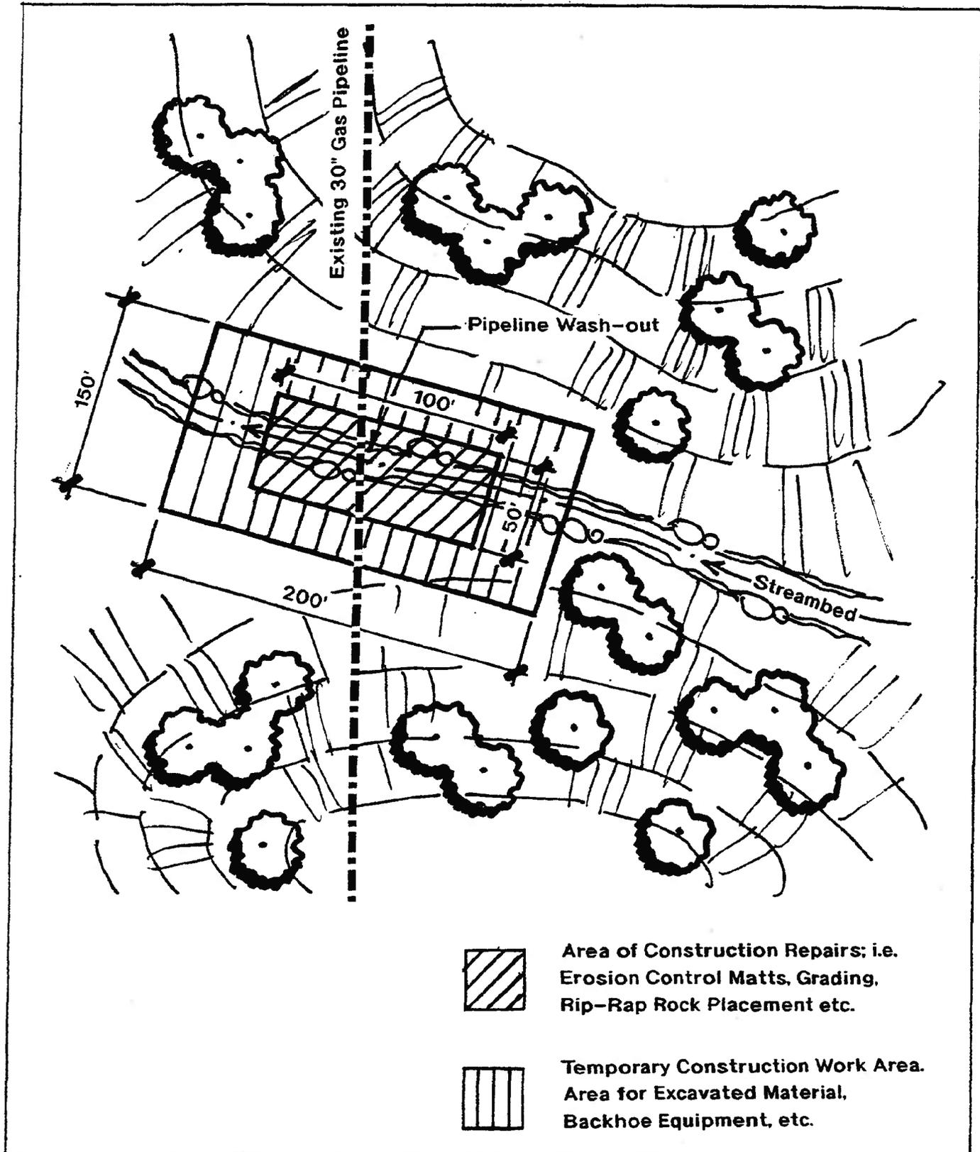
**Typical Corrective Streambed Repair
