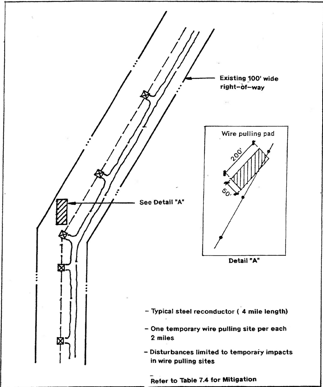
**Typical Electric Transmission Reconductor
