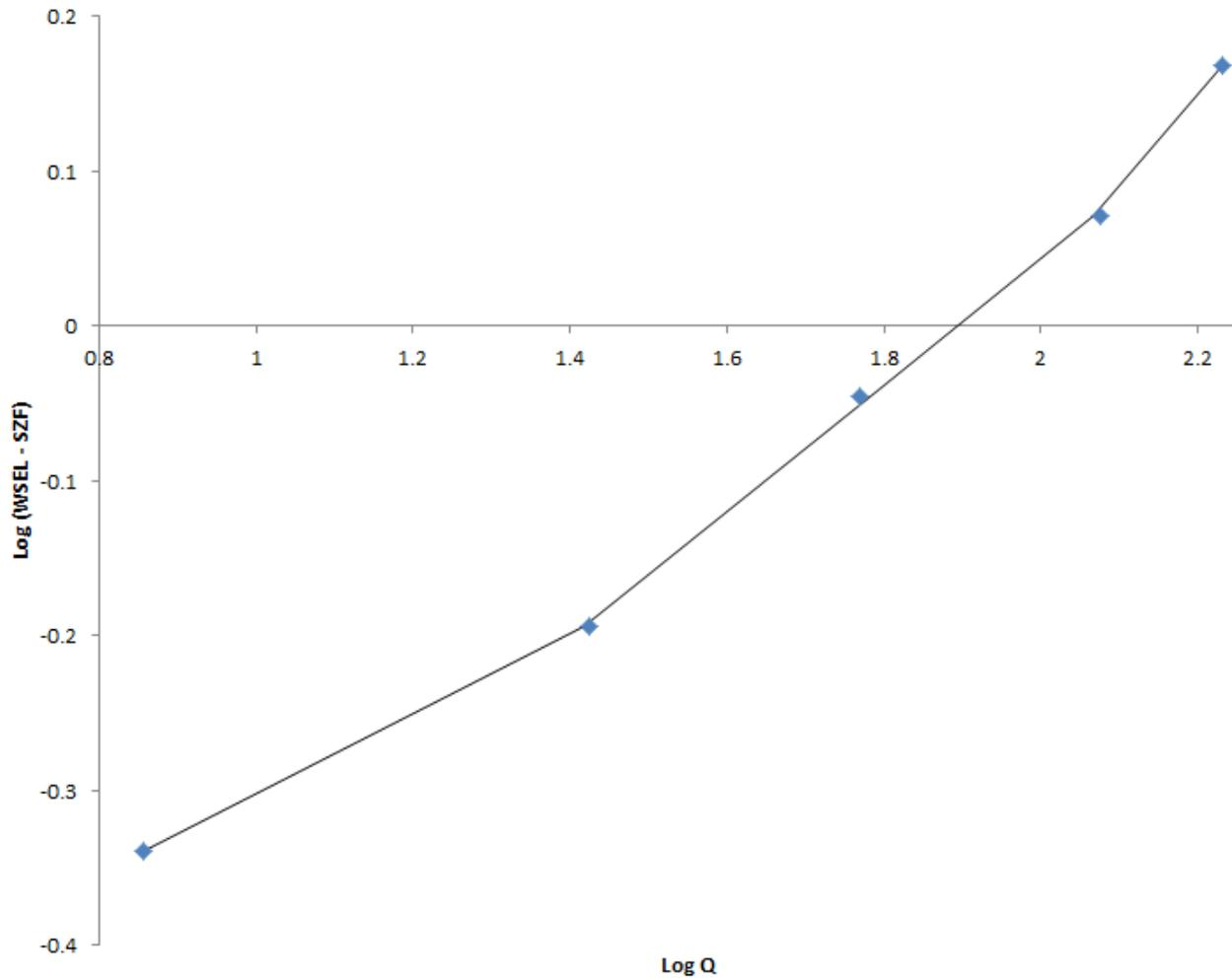
Figure 37. Lahar site 2015 pressure transducer rating curve.
