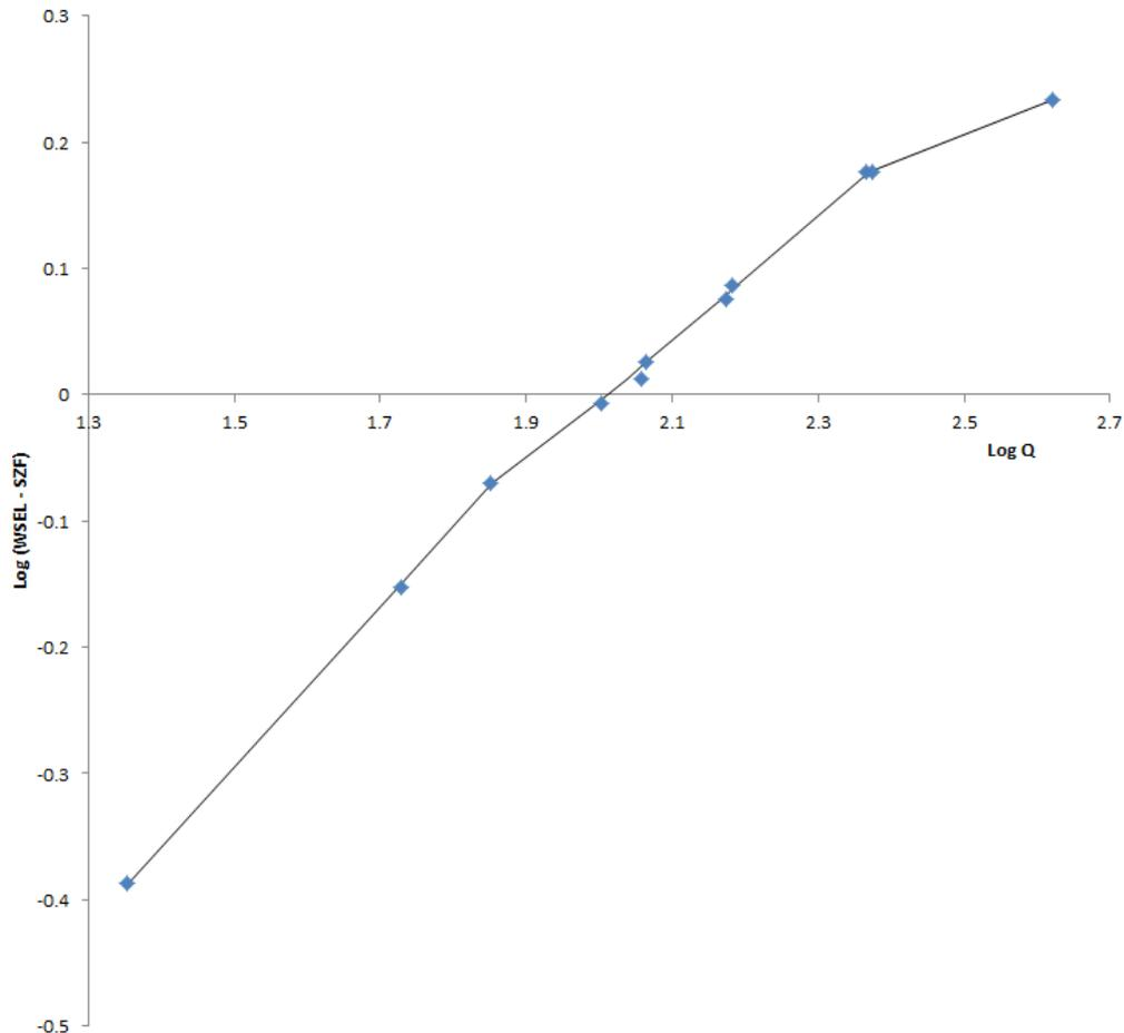
Figure 36. Lahar site 2014 pressure transducer rating curve.
