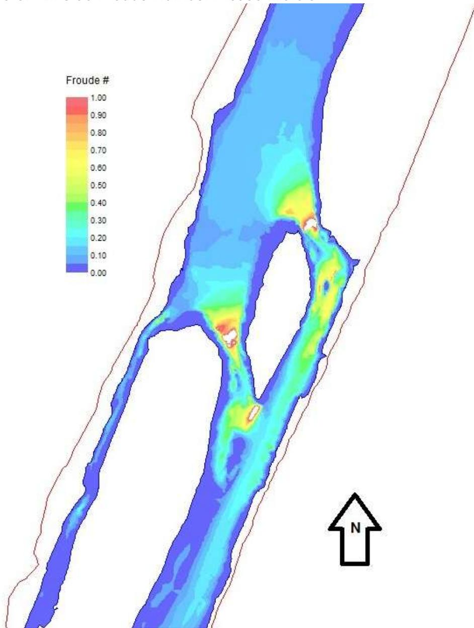
Figure J-4. Riffle 97 Froude Number Plot at 390 cfs.
