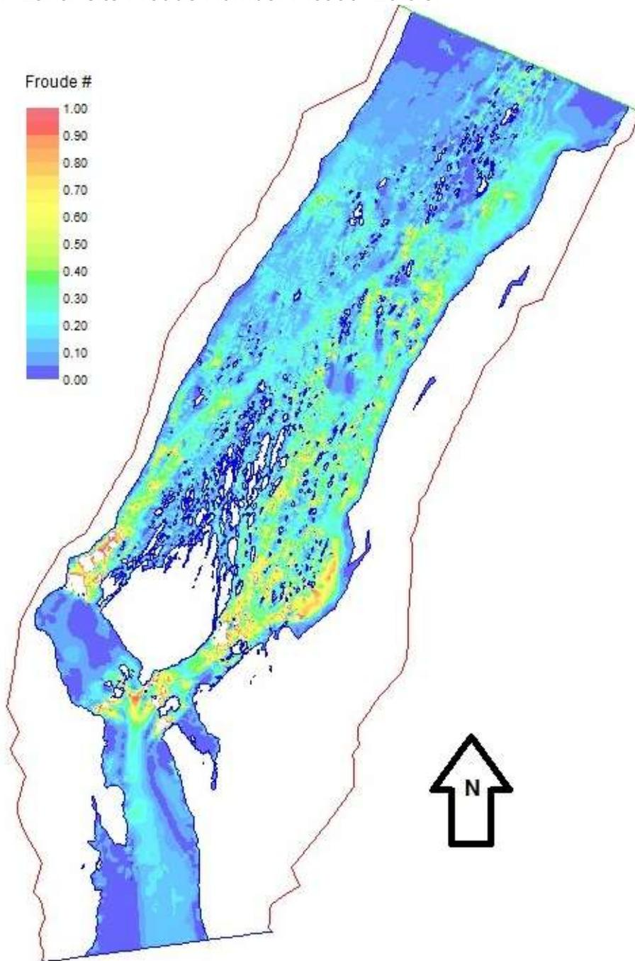
Figure J-2. Riffle 95 Froude Number Plot at 200 cfs.
