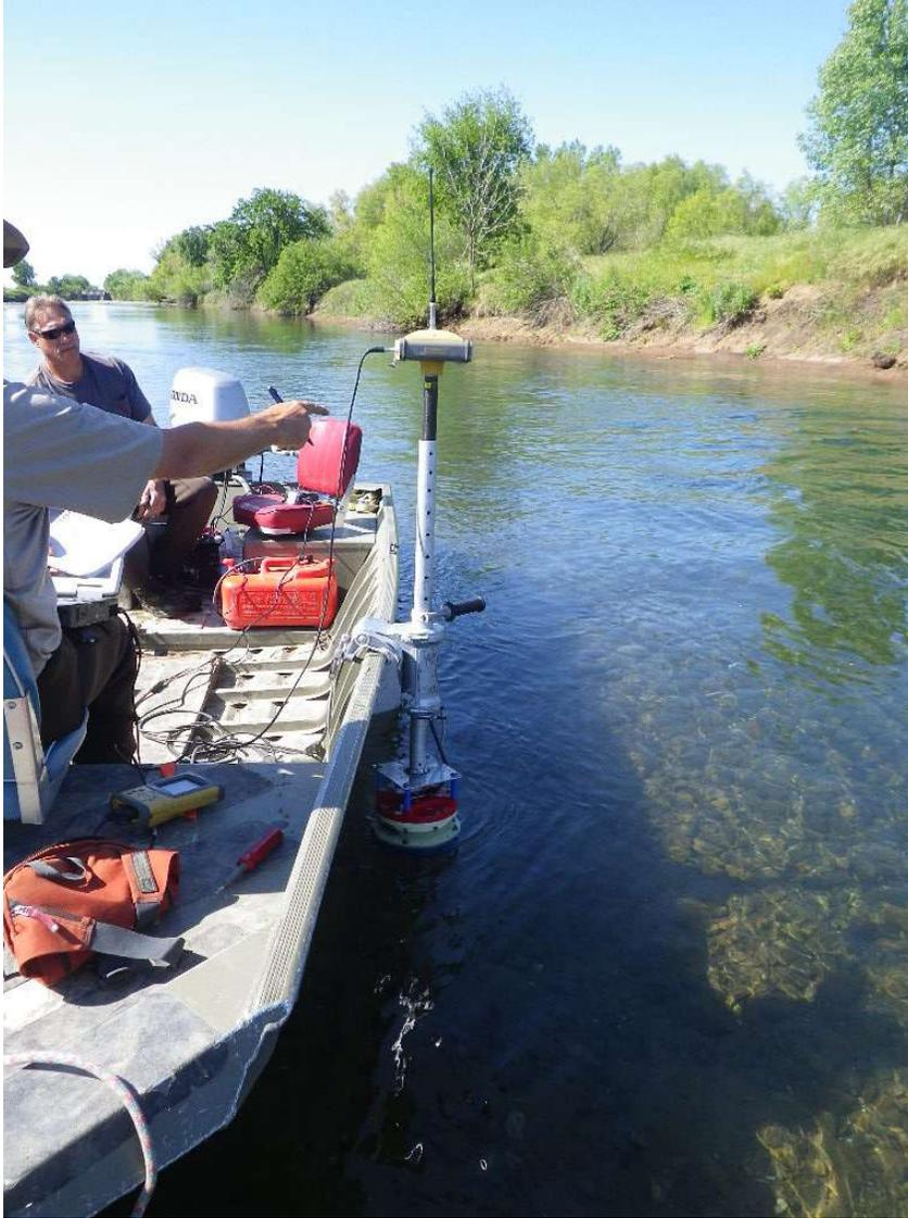
Figure 22. Boat-mounted ADCP.
