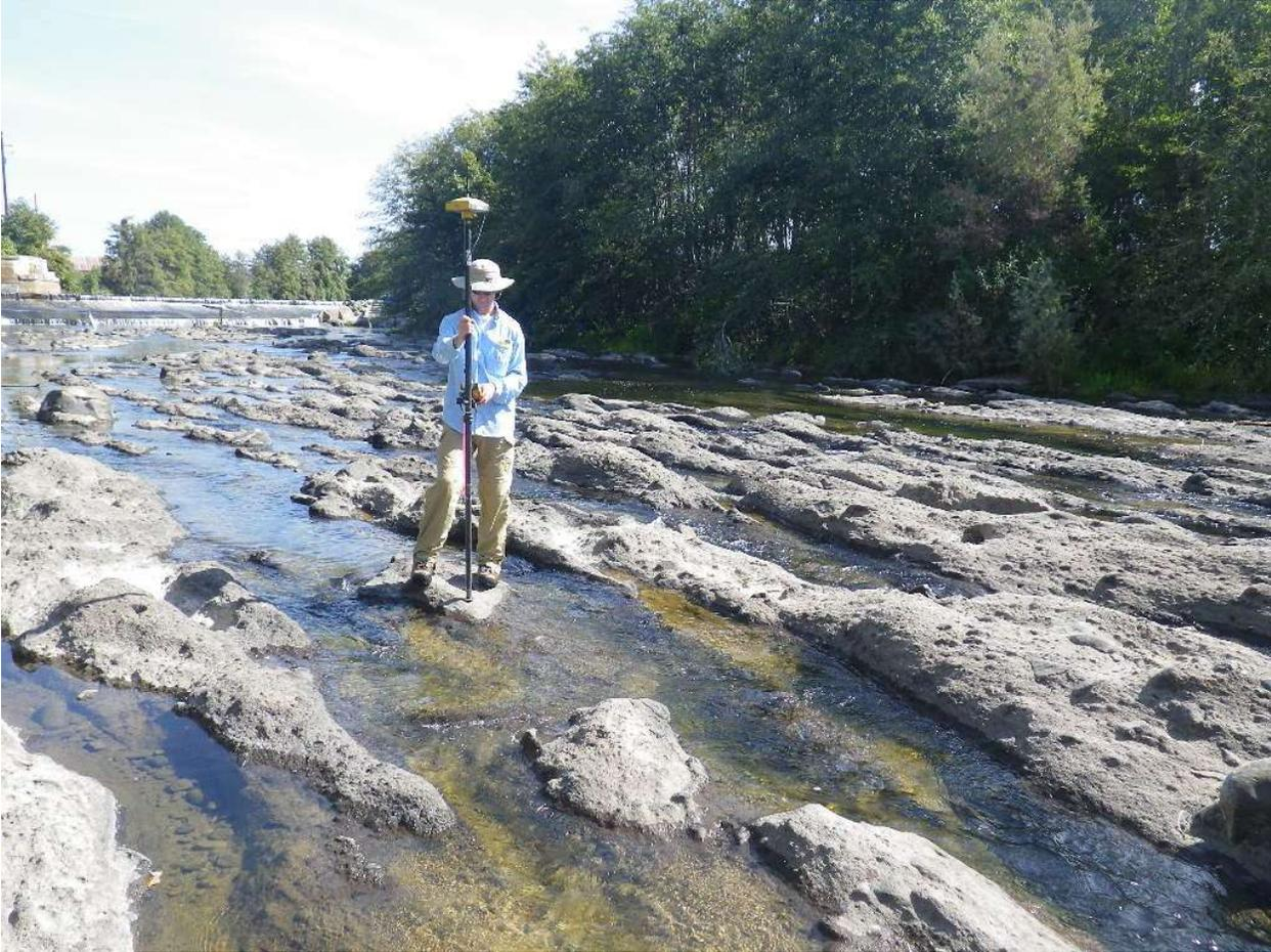
Figure 20. RTK GPS survey of Lahar Site.
