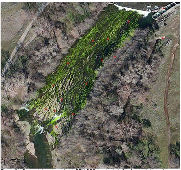
Figure 21. Data points collected with RTK GPS and total station (green dots) and control points used for terrestrial LIDAR (red points) for the Lahar site.
