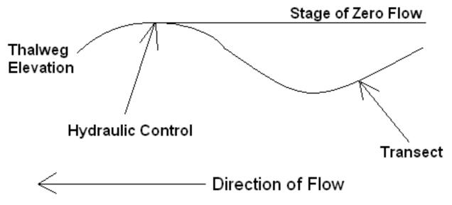
Figure 23. Stage of zero flow diagram.
