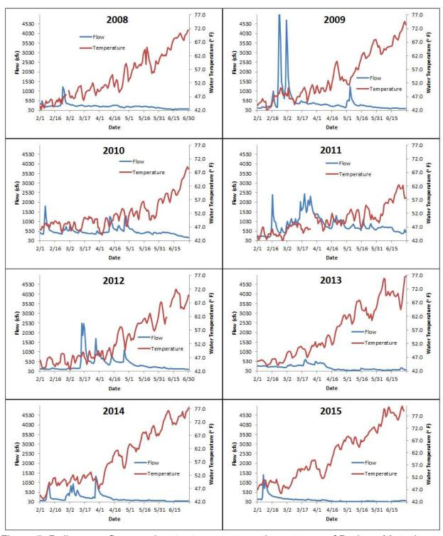
Figure 5. Daily mean flows and water temperatures downstream of Durham Mutual Dam.
