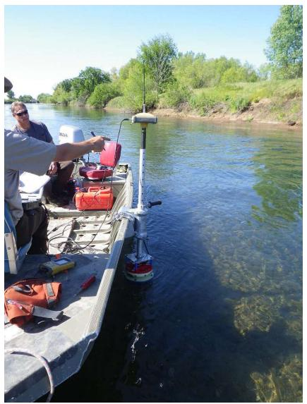
Figure 22. Boat-mounted ADCP.
