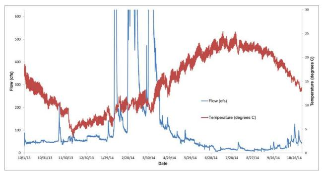
Figure 38. Water temperatures and flows at the Lahar in 2014. Gaps in the flow curve reflect flows that exceeded the upper end of the 2014 rating curve (630 cfs).
