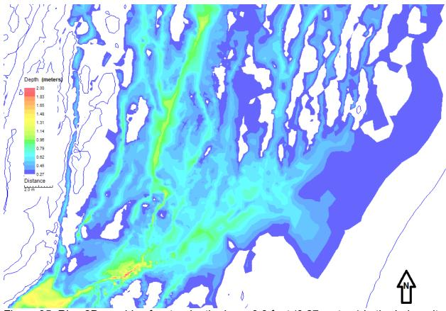
Figure 35. River2D graphic of water depth above 0.9 feet (0.27 meters) in the Lahar site at 405 cfs. The limiting width was equal to approximately 7.5 feet. Scale in meters.
