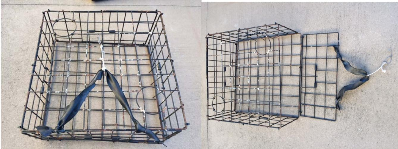
Box Trap using rubber strap, single strand No. 120 untreated cotton twine, and hook to secure side of trap. When No. 120 untreated cotton twine deteriorates, the open side of the trap meets 5" diameter destruct device.
