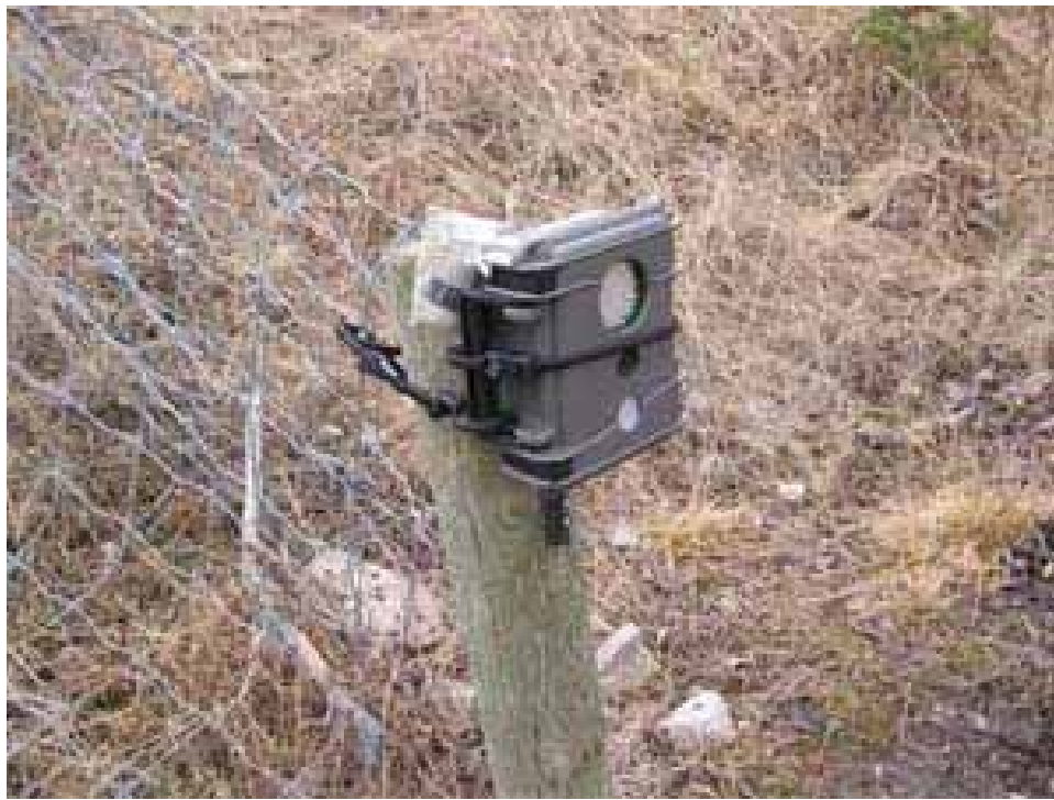
Figure 75. Photo. Remote digital infrared-operated camera (Credit: Tony Clevenger/WTI).
