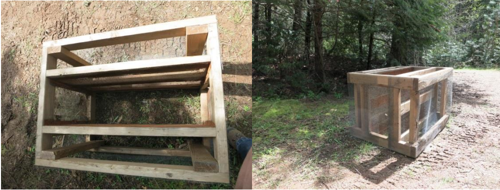
This screen is suitable for Class II watercourses and was brought for demonstration purposes by Sierra Pacific Industries to the Rancho Cordova Water Drafting Workshop, April 2016
