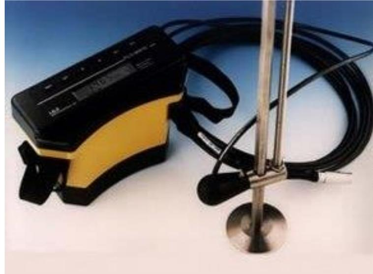
For use on stream channels with depths greater than 3 inches (~ 8 centimeters) and velocities greater than 0.01 feet per second.
