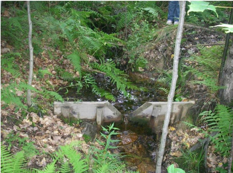
For use on small stream channels with depth where other methods are not feasible, or a high degree of accuracy is required (Flow studies).
