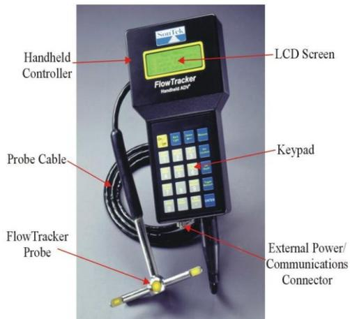
Measures **velocities** with a range as low as **0.001 m/s (0.003 ft/s)** and up to **4.5 m/s (15 ft/s)**.
