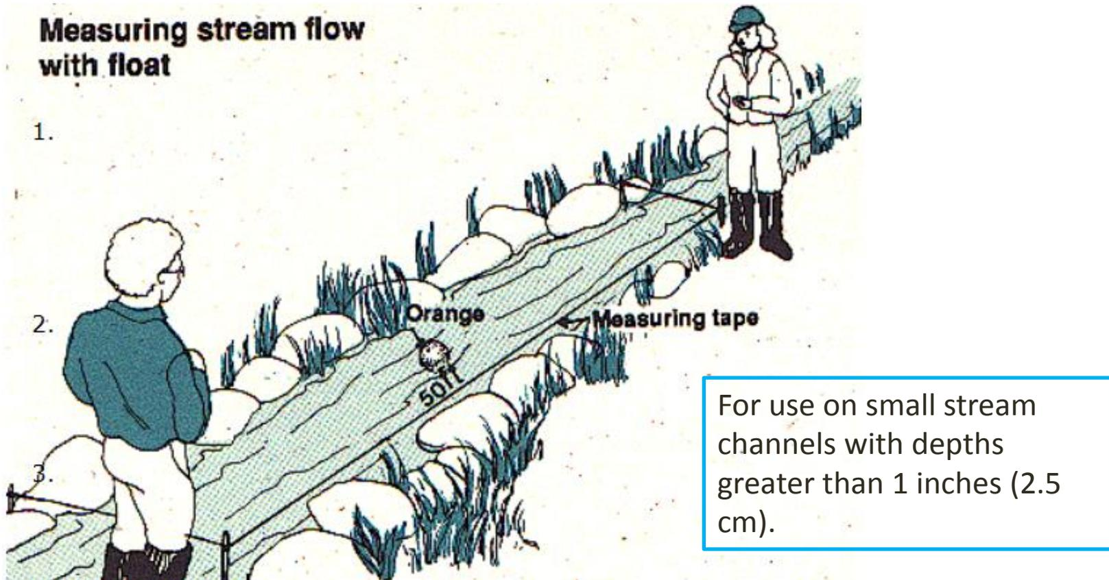
Because surface velocities are typically higher than mean or average velocities  $V_{\text{mean}} = k V_{\text{surface}}$  where  $k$  is a coefficient that generally ranges from 0.8 for rough beds to 0.9 for smooth beds (0.85 is a commonly used value)
