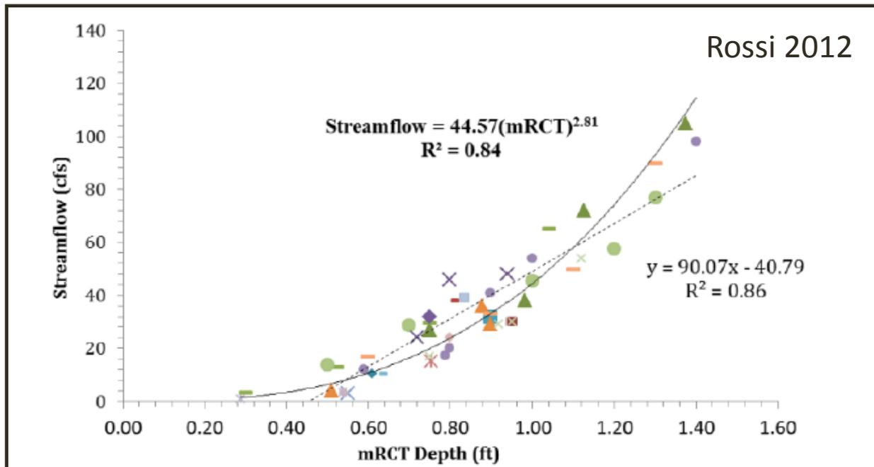
For use on larger streams with riffle crest depths greater than 3 inches or flows greater than 2 cfs.
