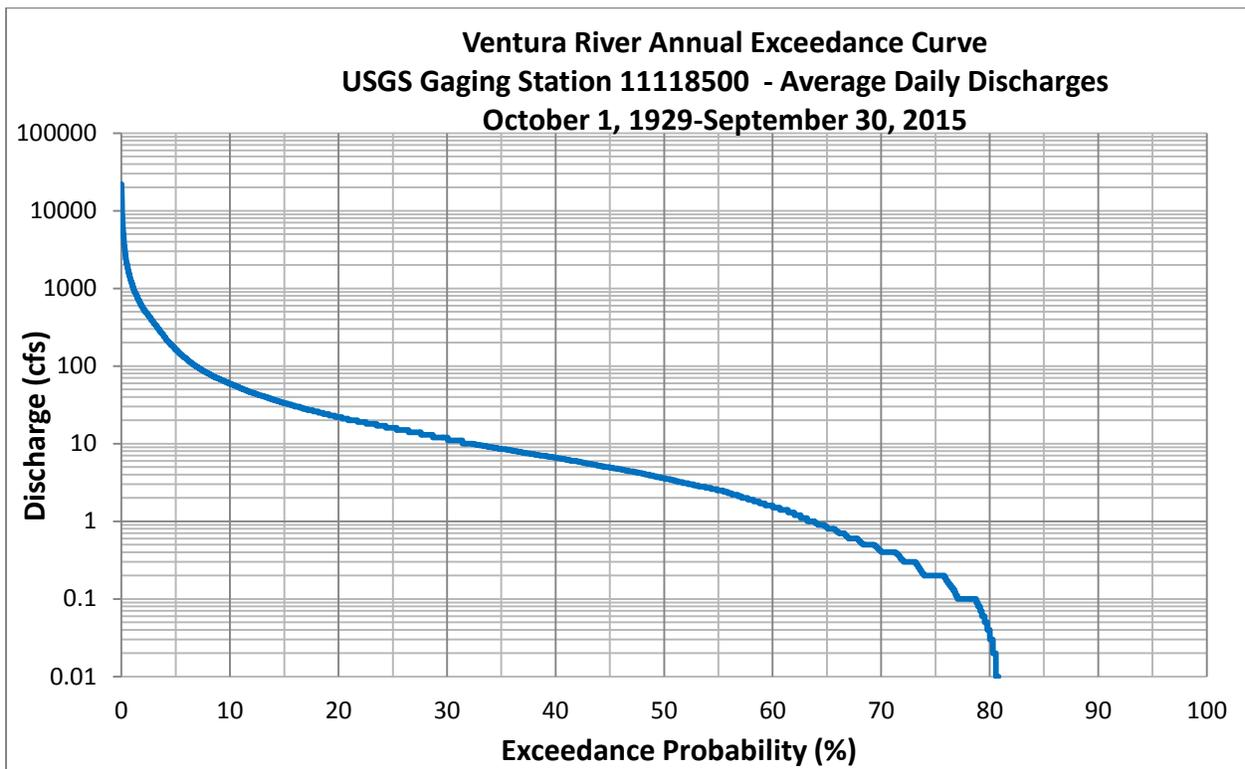
Figure 5. Annual Exceedance Flows for USGS Gage Station 11118500 Ventura River near Ventura from October 1, 1929-September 30, 2015
