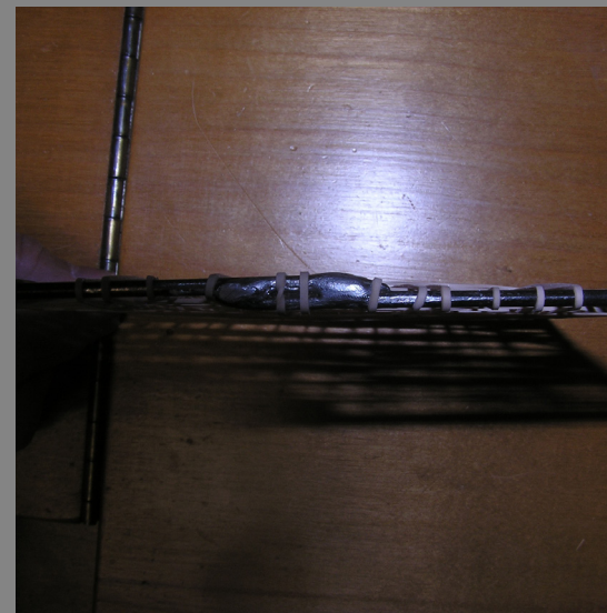
Photo 2: Overlap of wire frame, with soldered & filed smooth ends.
