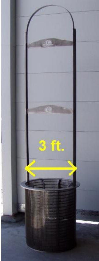
Figure 4 – One of the eight strainer baskets.
