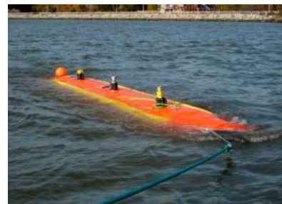
Fig. 17 Towable oil tank
