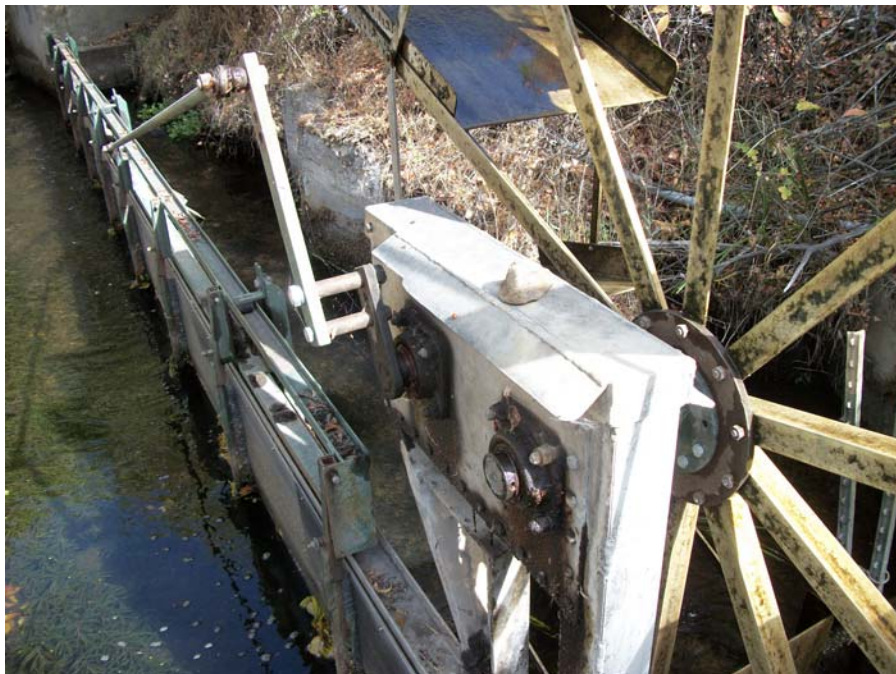
Site HR02. Roll Hart-01, Frame 14. Water wheel mechanism where it connects to fish screen. View 80 degrees. 9/30/2016.
