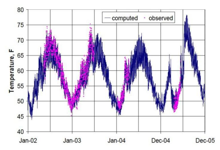
Figure C.4: Computed and observed temperatures at Sportsman Club (12 miles D/S). Originally Figure 3-18 in Resource Management Associates, Inc. (2007)
