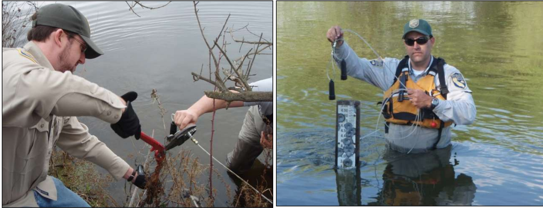
Figure 8: CDFW scientists installing temperature data loggers in the San Joaquin River
