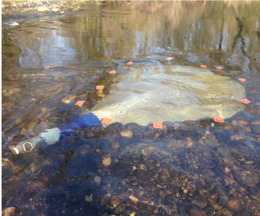
Figure 6: Emergence trap installed in winter 2015 to observe fry emergence from a Chinook salmon redd
