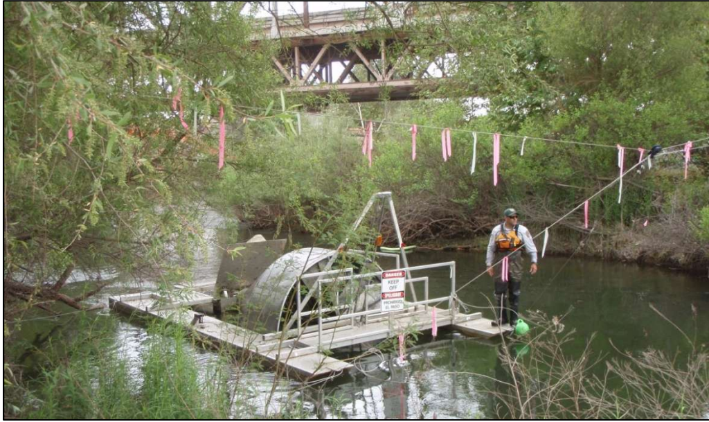
Figure 14: Rotary Screw Trap operated near the Hwy 99 Bridge
