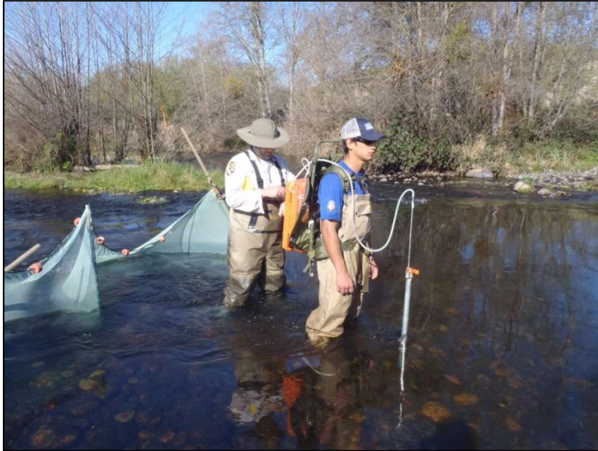
Figure 13: CDFW and AmeriCorps staff measure intragravel flow within a fall-run 2014 Chinook Salmon redd
