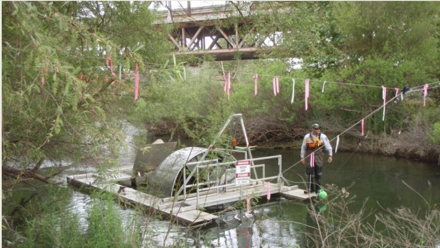
Rotary Screw Trap for monitoring survival and migration of juvenile Chinook Salmon
