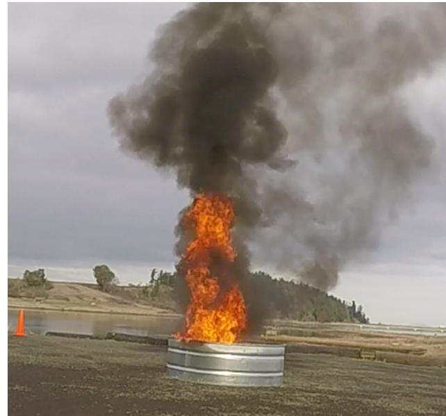
500 mL oil with sea ice and 1/10 aggregator Higher intensity burn
