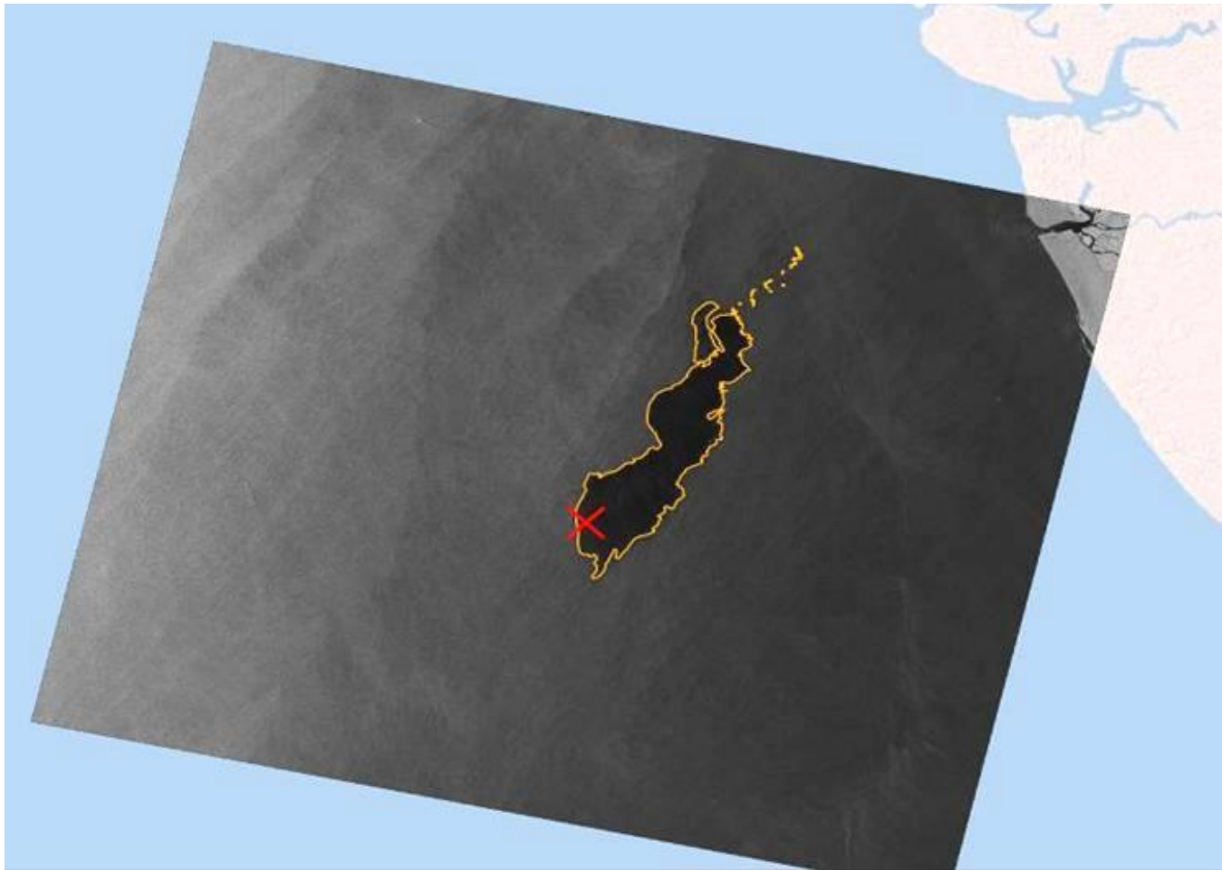
Dec 21 RADARSAT-2 ScanSAR Narrow (50 m res) (05:52 UTC) Oil on ocean surface for 18 hrs.
