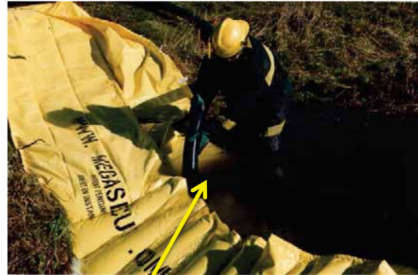
Instant UnderFlow dam for mechanical skimmers & vacuums
