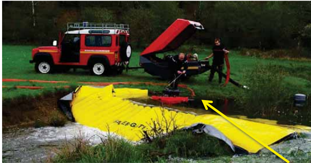
Instant UnderFlow dam for mechanical skimmers & vacuums
