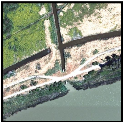
Non-tidal, smaller waterways and graded or maintained permanent or temporary ditches that may or may not contain water at the time of the imagery.
