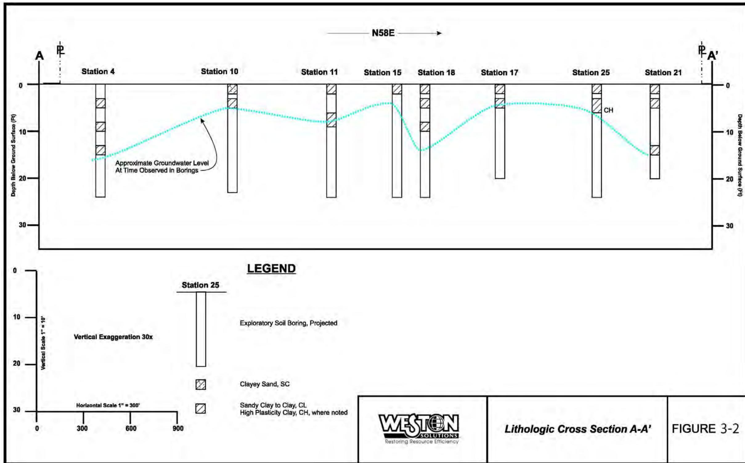
Figure 3-2. Cross Section A-A'
