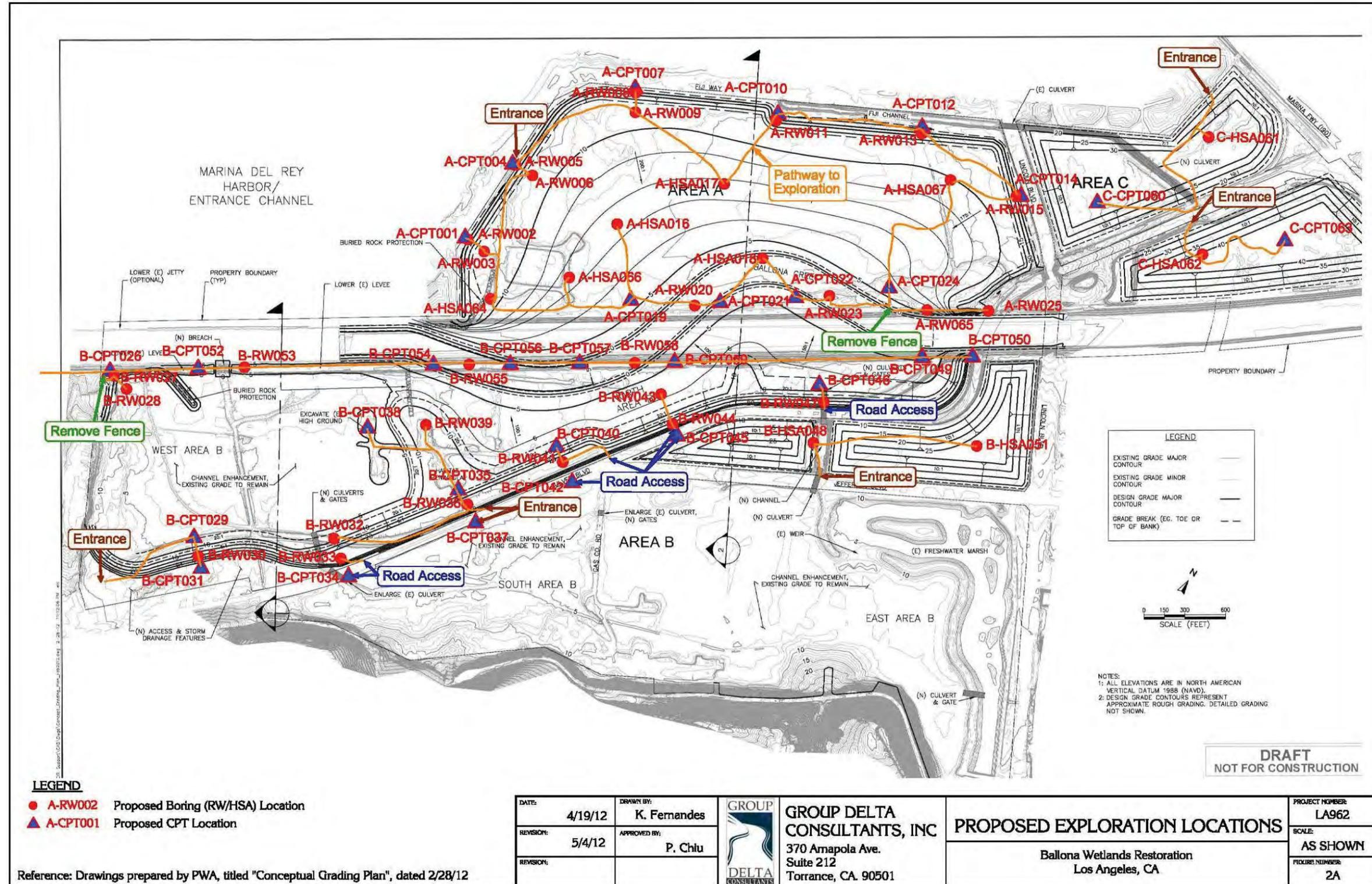
Figure 2-1. Proposed Geotechnical Investigation Boring Location Plan (Group Delta)
