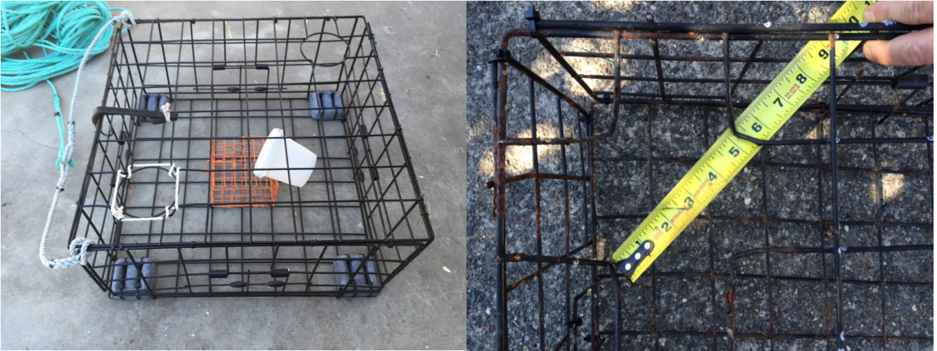
#1-Box Trap with single strand No. 120 untreated cotton twine attached to 4 1/4" Escape Ring. #2 – Escape Ring removed. Corners of attachment points to the Escape Ring are bent down to achieve 5" diameter destruct device.
