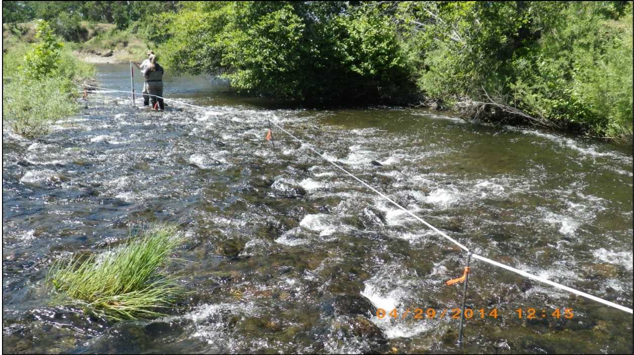
Figure 9. Critical riffle analysis transect along the shallowest course from bank to bank at riffle CR31 in lower Deer Creek. Photo looking downstream.
