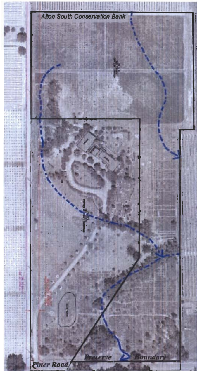
Figure 2. Surface drainage patterns at Alton South Conservation Bank.
