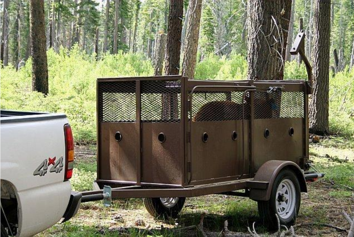
Figure 2: Bear Trap; trap is set by opening the back, luring bears in with bait, when the bear pulls on bait bag attached to a cable running through the conduit and work the trigger. The round portholes on all sides provide access by jab stick.
