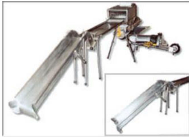
Figure 34. Access ramp manufactured by Talleres Aguin. The ramp is placed overboard and the mussel ropes are pulled up the ramp by the hauler.
