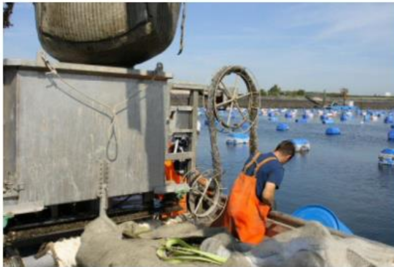
Figure 33. A New Zealand continuous seeding machine from Bakker in the Netherlands
