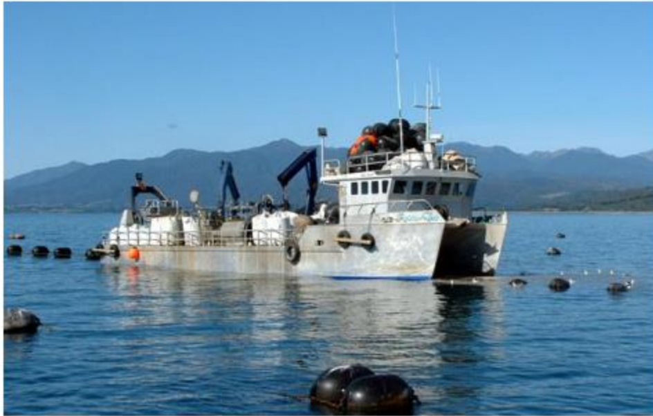
Figure 44. A catamaran harvest vessel in New Zealand with 1 ton mussel containment bags for bulk storage and handling.
