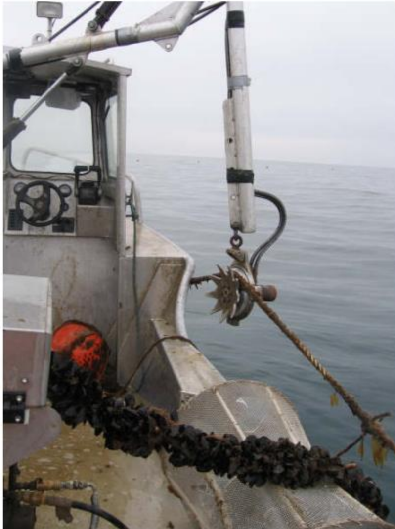
Figure 21. A hydraulically powered starwheel fixed to the end of a crane on a small mussel tending vessel. The starwheel also provides mobility along the line for tending the crop.
