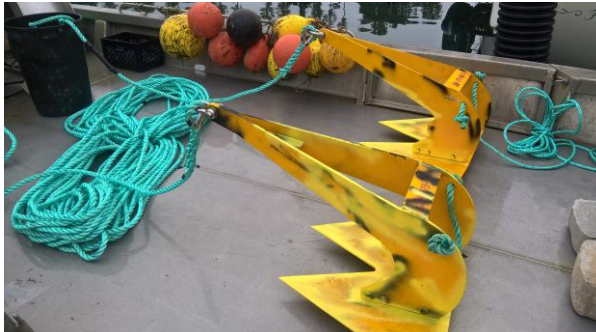
Jeyco Stingray anchors, 75kg, with one-inch co-polymer anchor rodes attached.
