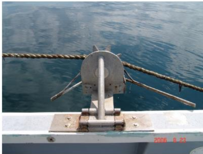
Figure 26. An example of an idler starwheel mounted on the aft portion of the rail of a service vessel.
