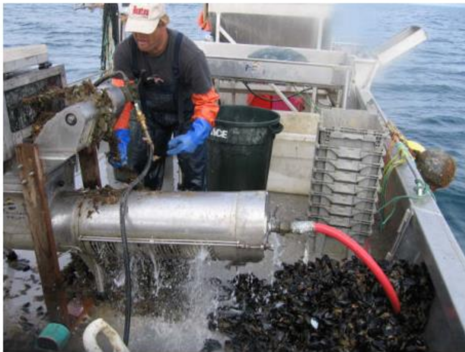
Figure 40. Photo of the Talleres Aguin declumper with seawater hose attached for washing the mussels
