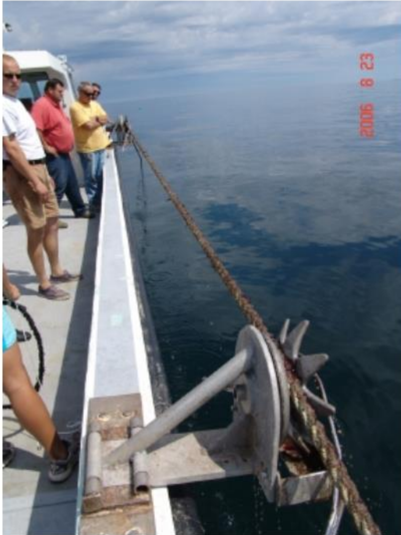
Figure 27. A photo of the backbone of a longline set into the aft (foreground) and forward starwheels (background).
