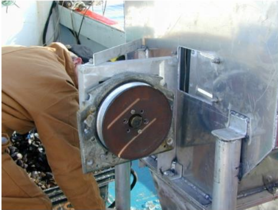
Figure 37. A rear view of the University of New Hampshire's harvesting machine showing the hydraulic hauler. The growing rope is pulled through the slot with stiff rubber flaps to the right of the hauler wheel.
