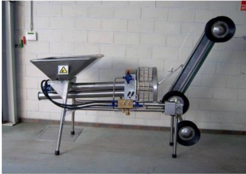
Figure 32. Continuous seeding machine model A6 manufactured by Talleres Aguin
