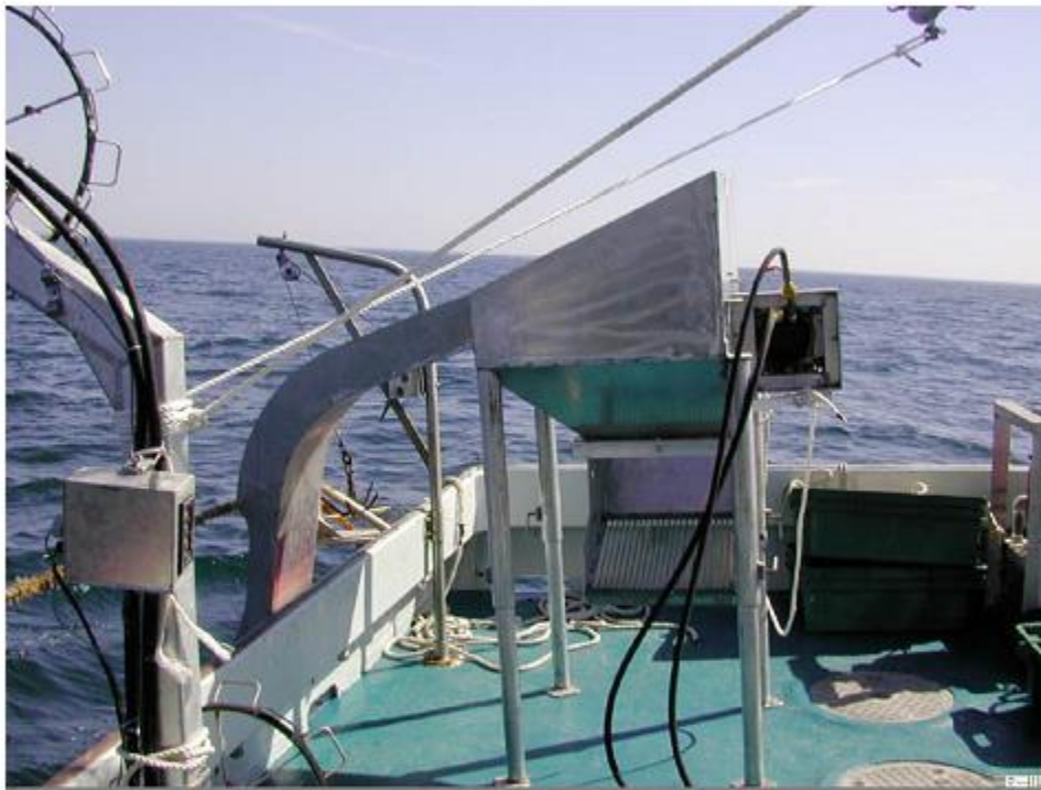
Figure 36. A mussel harvesting machine designed and built by the University of new Hampshire to harvest mussels from continuous New Zealand type growing ropes. The stripped mussels fall out of the bottom of the machine into containers or onto a conveyor belt.
