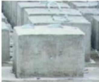
Figure 13: Concrete block with 2 rope loops embedded into the concrete (on top). The rope is tied to the internal rebar supports. Note that the block geometry shown here should not be utilized with this design, as it can be susceptible to tipping.
