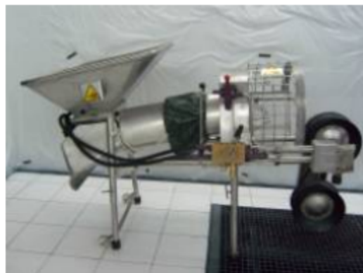
Figure 28. Model A4 seeding (tubing) machine for pegged rope manufactured by Talleres Aguin
