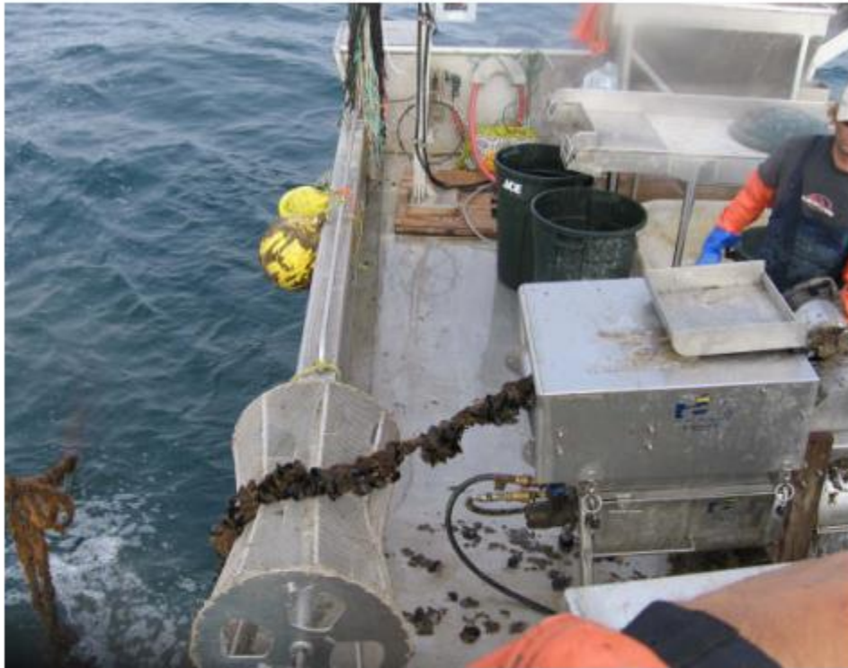
Figure 38. A rail mounted roller used in place of an access ramp. The mussel rope is pulled through a brush stripper. The hauler and stripper are mounted directly above a declumper. The machinery is manufactured by Talleres Aguin.
