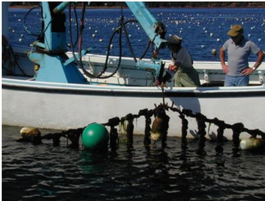
Figure 20. A mussel service vessel in PEI Canada with a hydraulic hauler fixed to the end of an articulating crane
