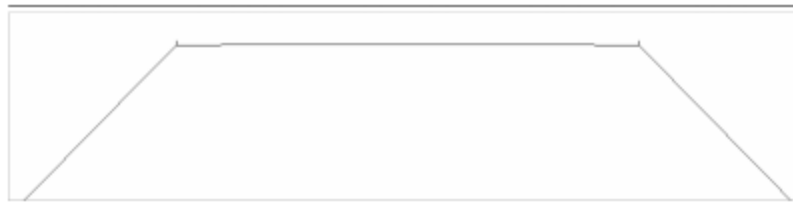
Figure 2: The deformed, steady state geometry of the long line system without mussel ropes.
