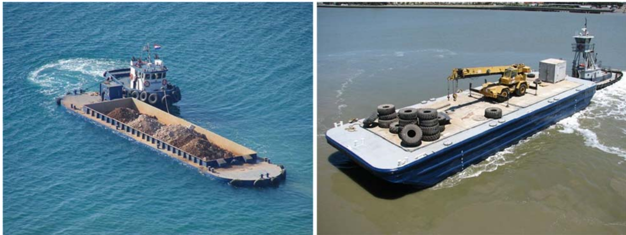
Figure 5-3: Hopper Barge (Left), Deck Barge (Right)
