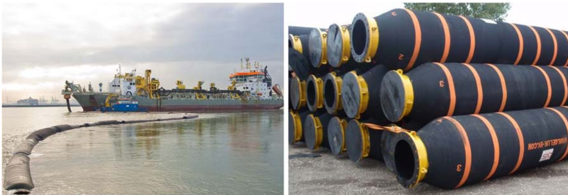
Figure 4-2: Slurry Pipeline System using floating hoses
