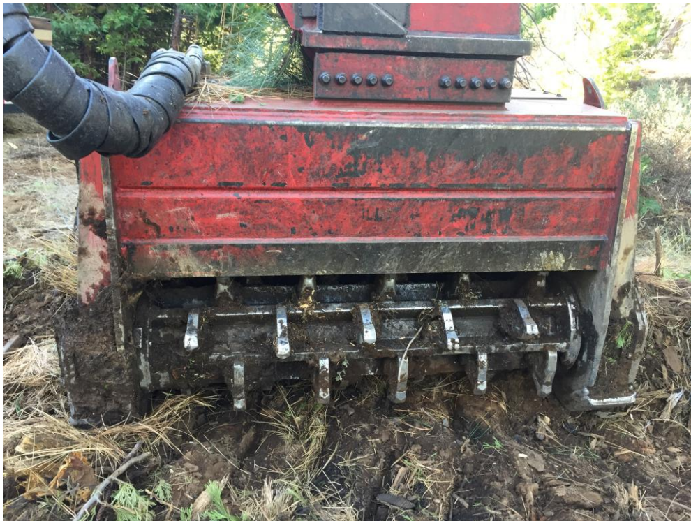
A close-up shot of the masticator head.
